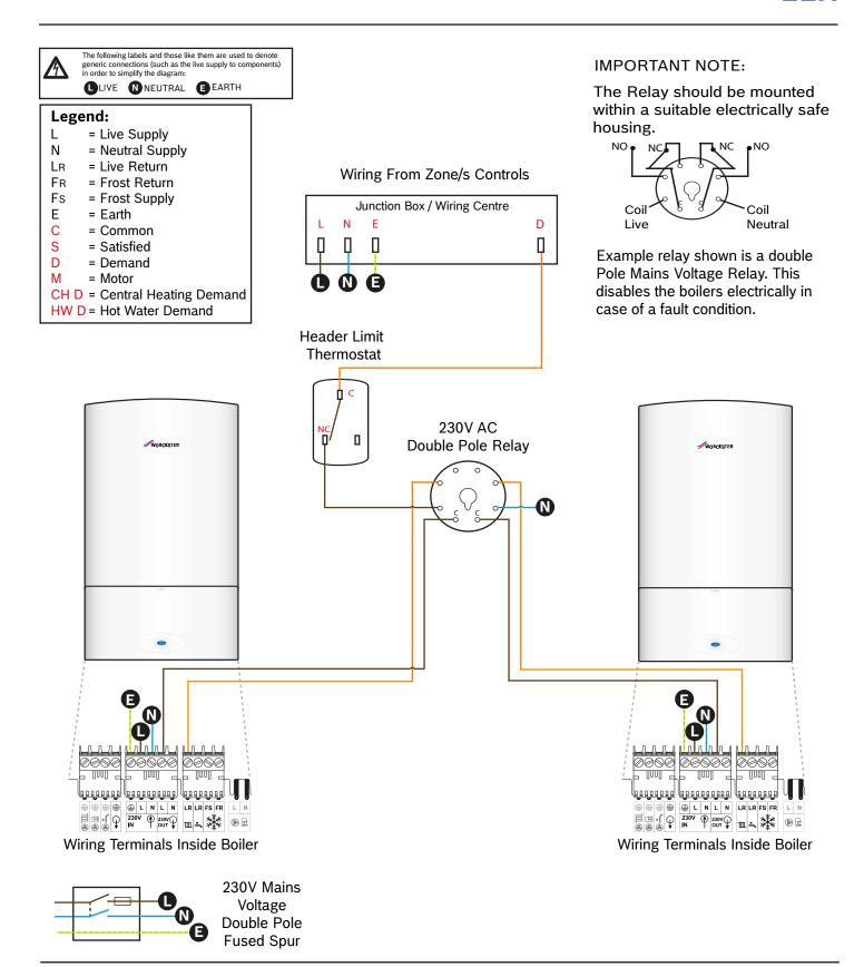
All electrical work should be carried out by a registered engineer. Wiring must comply with the latest IET wiring regulations.
