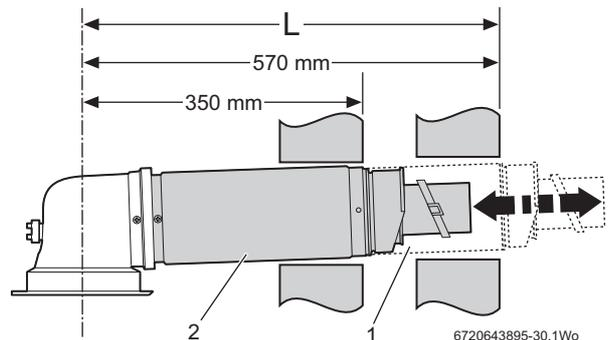
Fig. 8 Standard telescopic flue
