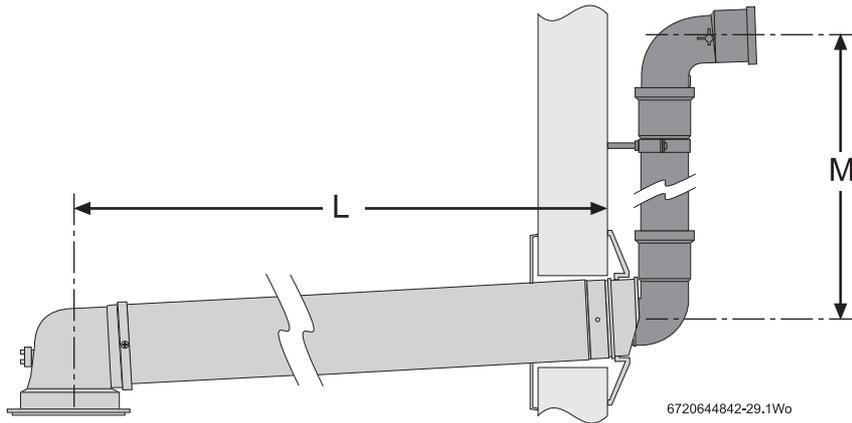
Fig. 32 Effective lengths L and M
