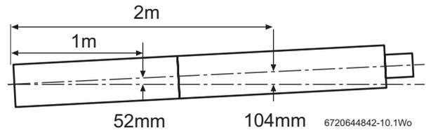
Fig. 20 Slope for condensate disposal
