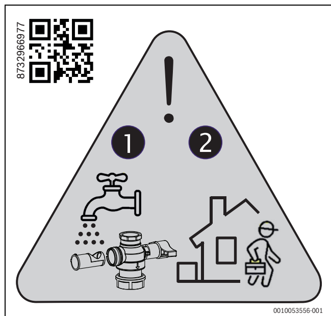
Fig. 55 Clean the particulate filter after maintenance
