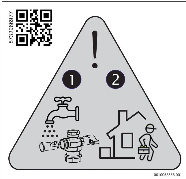
Fig. 43 Clean the particulate filter after commissioning and maintenance
