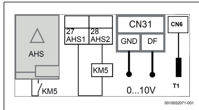
Fig. 91 Additional boiler
