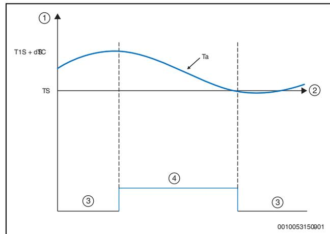
Fig. 122 Cooling mode - Air temperature ( $T_a$ )
