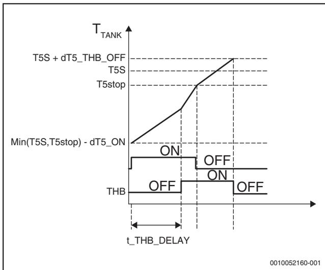
Fig. 117 Activation logic of the DISINFECT (anti-legionella) function
