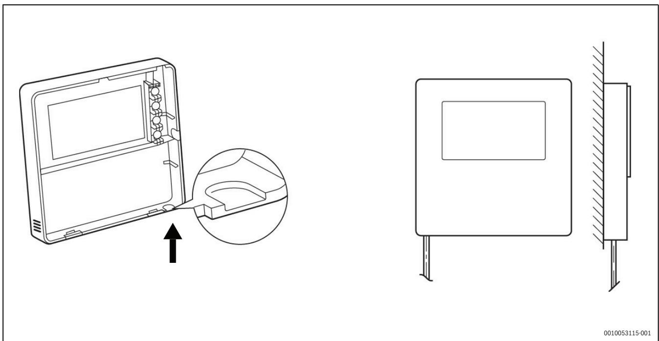
Fig. 95 Positioning of the cable outlet
