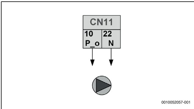
Fig. 81 External pump, type 2 control signal
