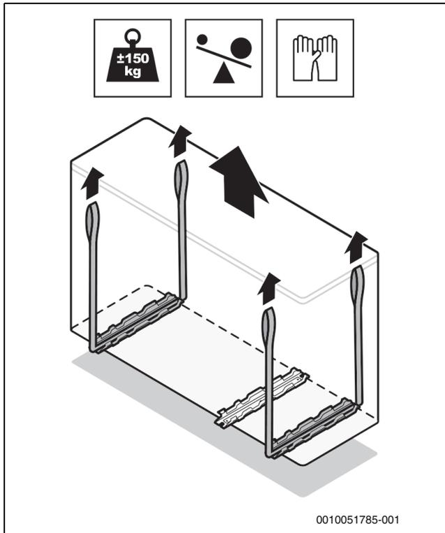
Fig. 44 Placing the unit
