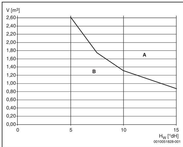
Fig. 52 Required limits for heat pump output < 50 kW
