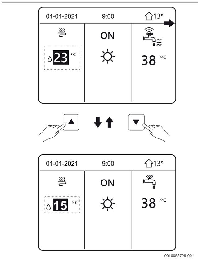
Fig. 172 Adjust temperature
