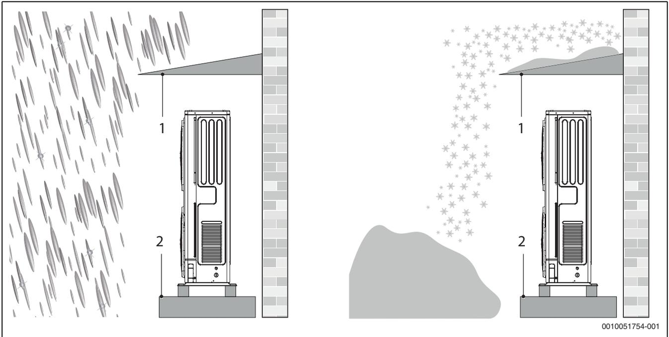
Fig. 39 Unit exposed to heavy rain or snow
