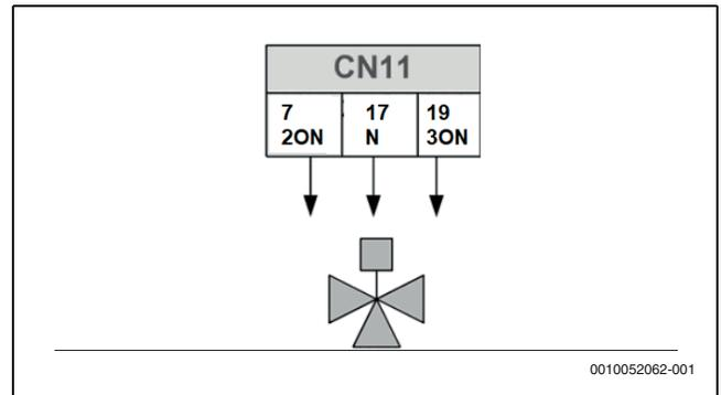
Fig. 85 3-way valve SV3, type 2 control signal
