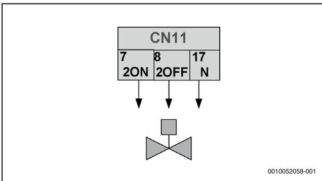
Fig. 82 SV2 2-way valve HMI configuration
