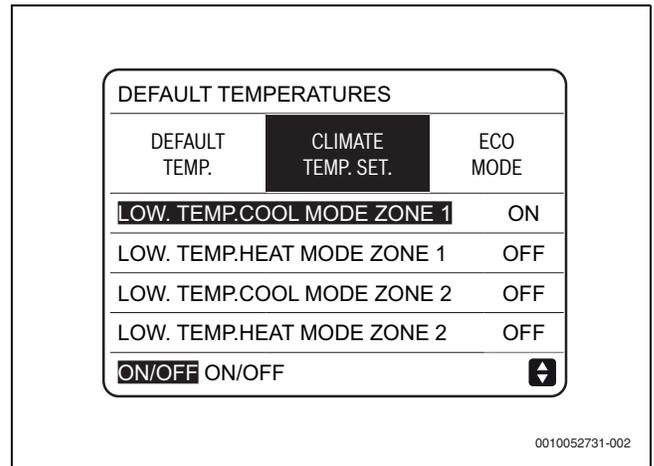
Fig. 181 CLIMATE TEMP. SET. is on
