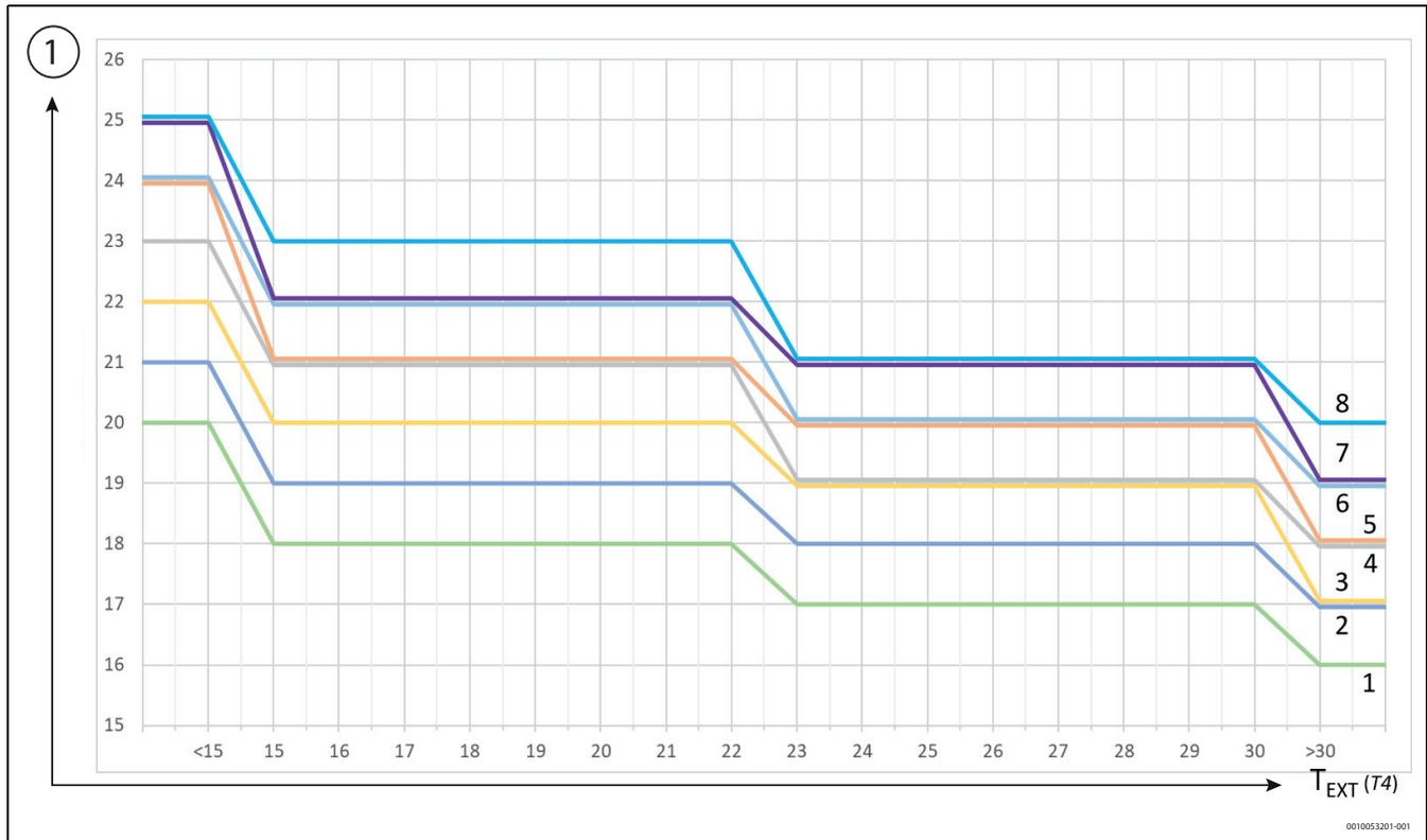
Fig. 147 Cooling mode on systems with radiant distribution
