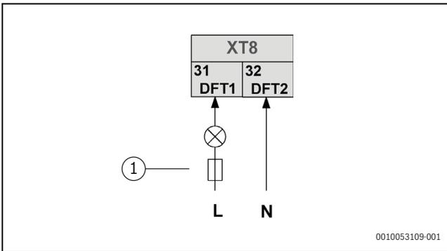
Fig. 89 Defrosting state or alarm state
