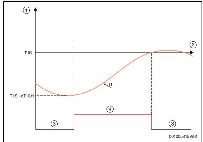
Fig. 124 Heating mode - Water supply temperature (T1)
