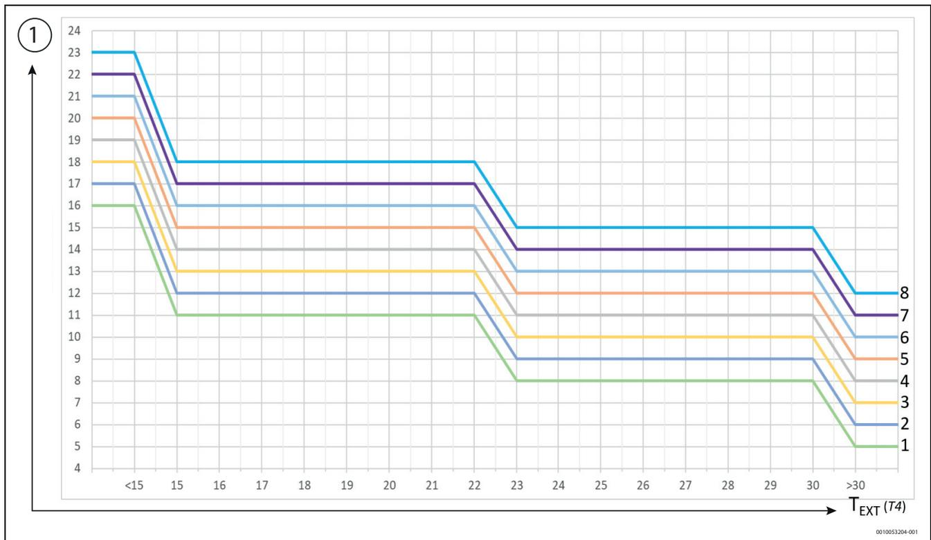
Fig. 148 Cooling mode on systems with terminal distribution
