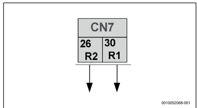
Fig. 88 Unit in operation signal
