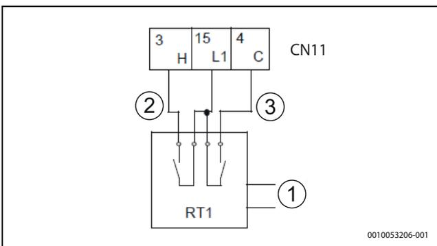
Fig. 100 Zone thermostat – Method A
