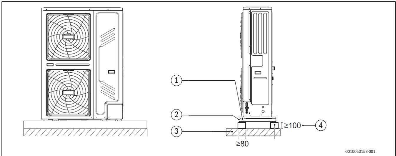
Fig. 42 Secure the unit with foundation bolts
