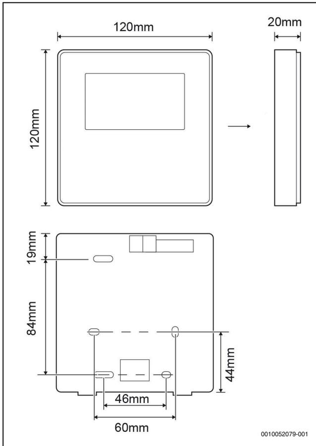
Fig. 94 User interface installation
