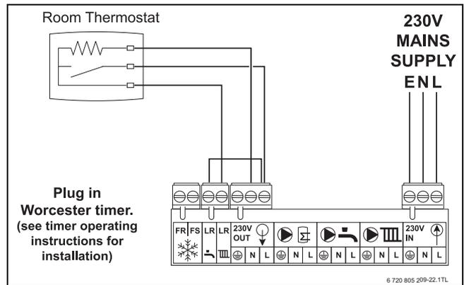
Fig. 45 Room Thermostat and Plug In Twin Channel Programmer
