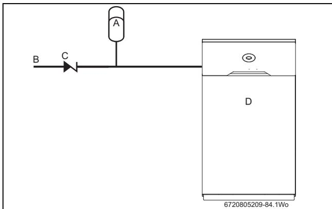
Fig. 3 Mains expansion vessel
