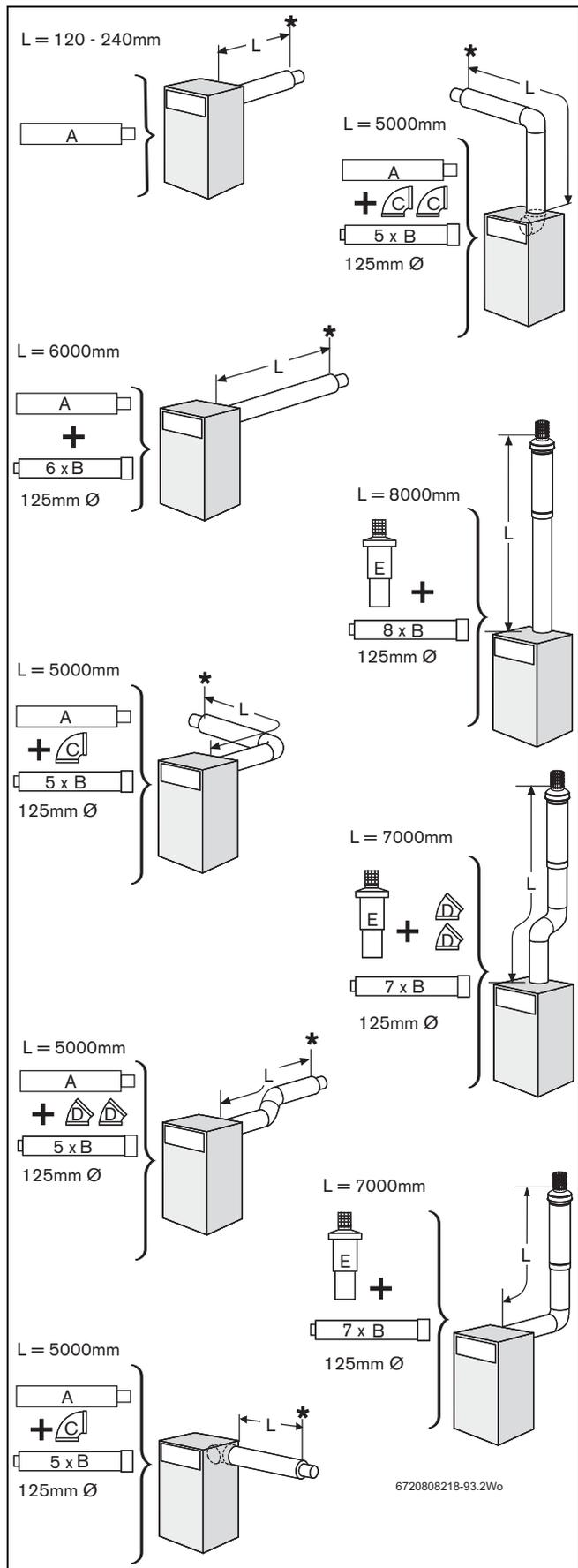
Fig. 24 Room sealed flue options
