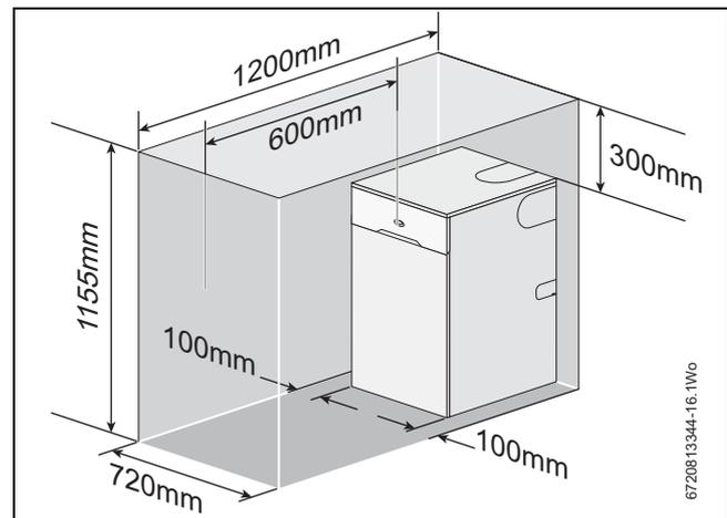
Fig. 19 Installation clearances
