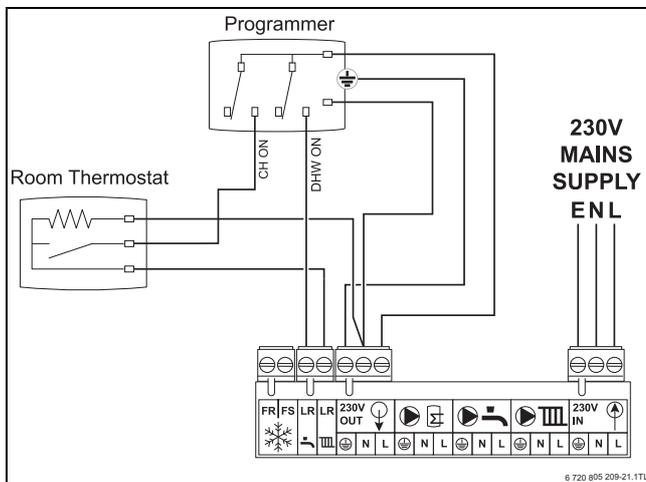
Fig. 44 External 230 V Twin Channel Programmer and Room Thermostat
