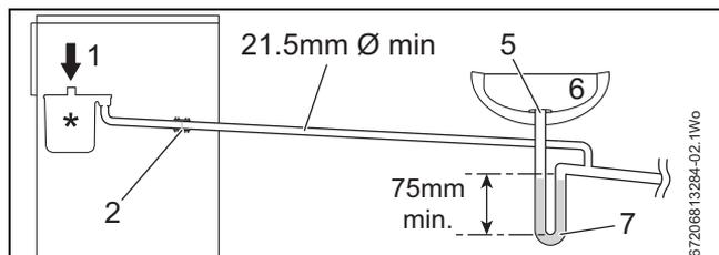
Fig. 12 Disposal to a waste pipe
