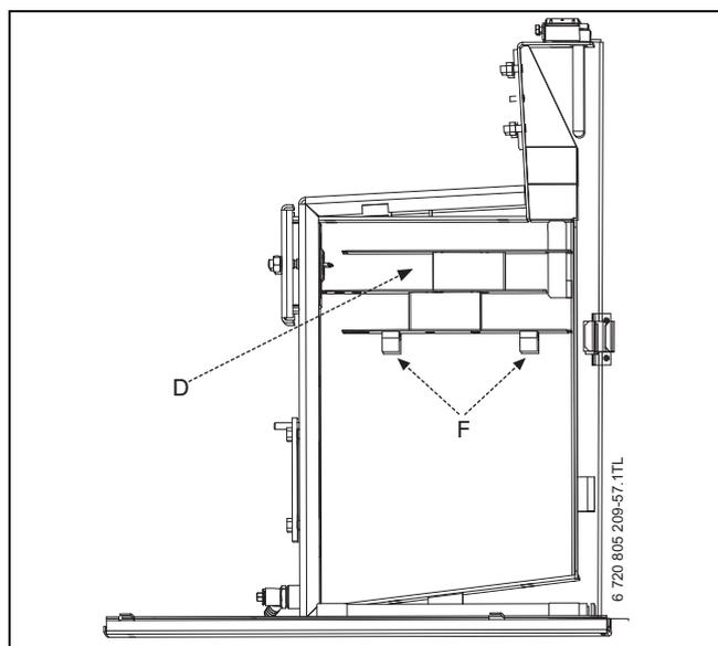
Fig. 81 Baffle location
