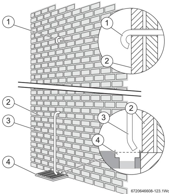
Fig. 18 Pressure relief pipe work
