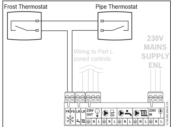
Fig. 46 Optional External 230 V AC Frost Stat Connection for protection of system pipework in unheated air space
