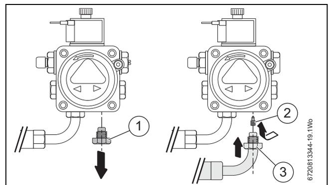
Fig. 38 Converting to double pipe system
