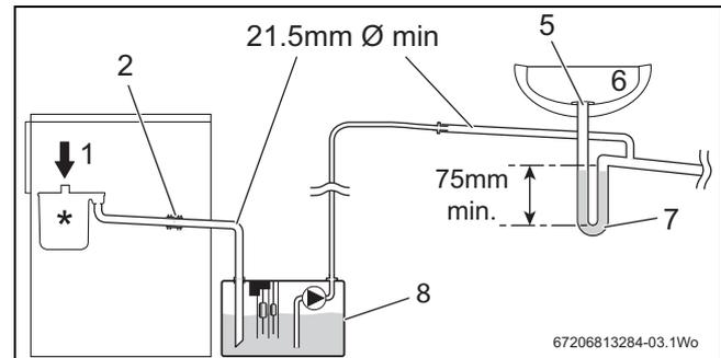
Fig. 13 Disposal via a condensate pump
