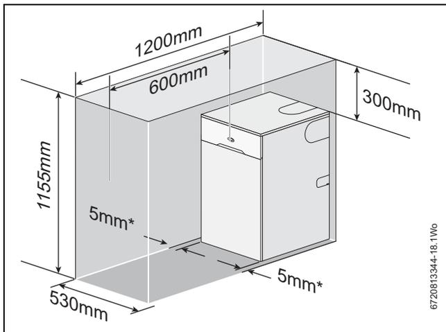
Fig. 21 Maintenance and repair clearances
