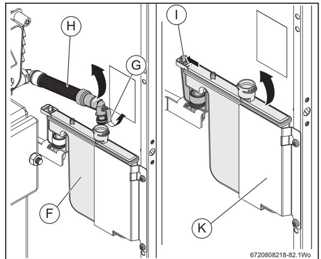
Fig. 78 Condensate trap detail
