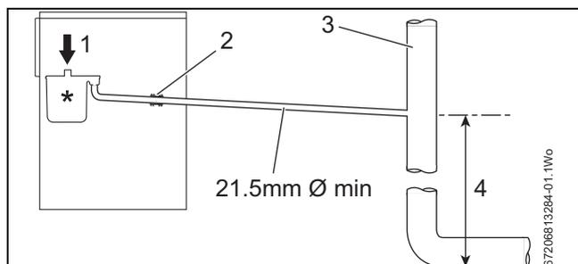
Fig. 11 Disposal to a soil vent stack
