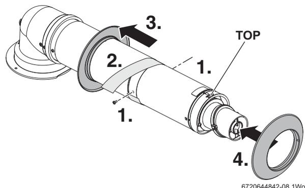
Fig. 40 Telescopic flue
