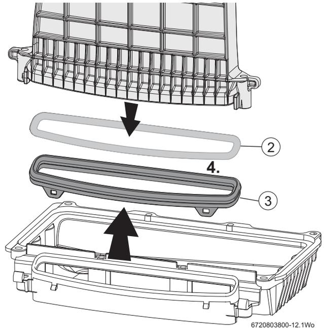
Fig. 92 Remove the existing seal
