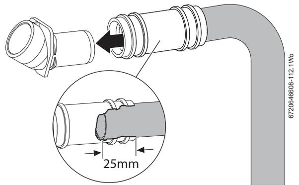
Fig. 28 Condensate connection
