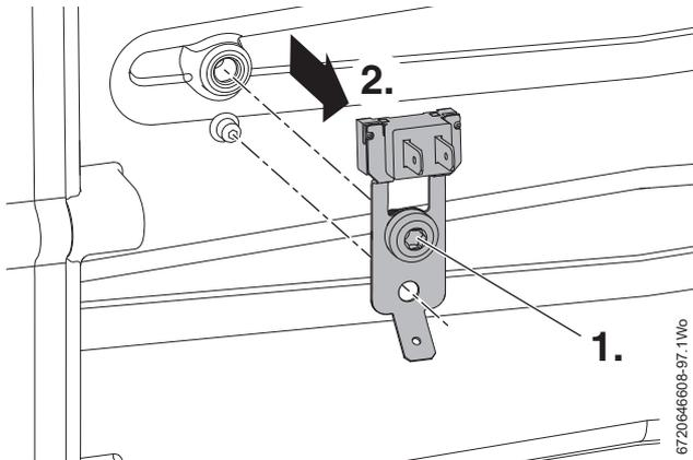
Fig. 87 Overheat sensor
