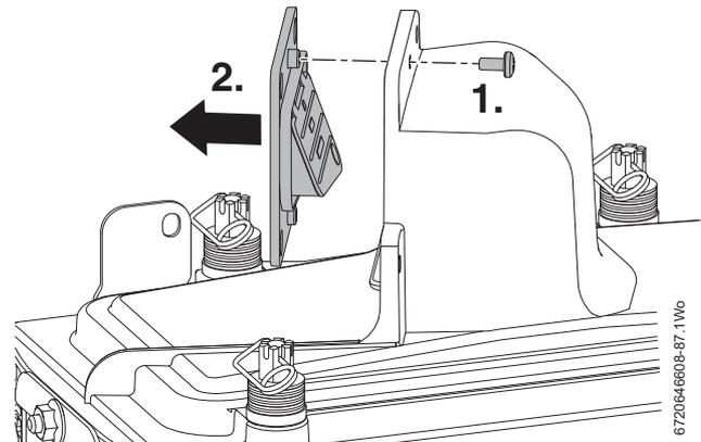
Fig. 98 Air/gas flap valve
