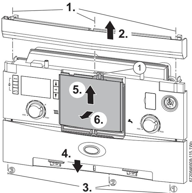
Fig. 49 Removing the blanking plate
