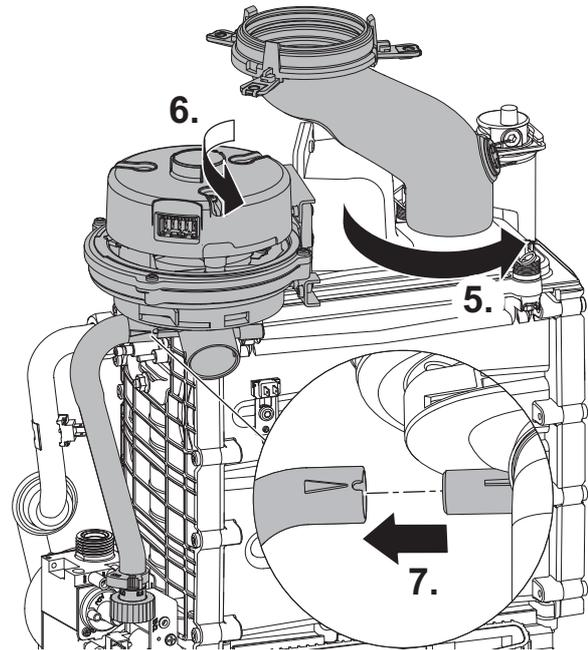
Fig. 97 Fan removal 2
