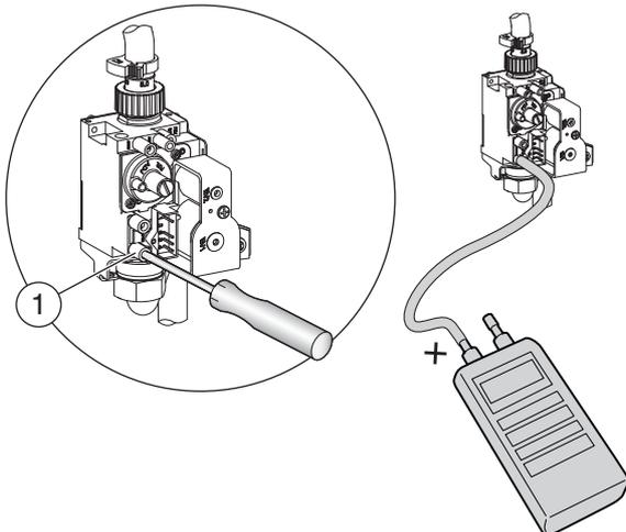
Fig. 59 Inlet pressure test point
