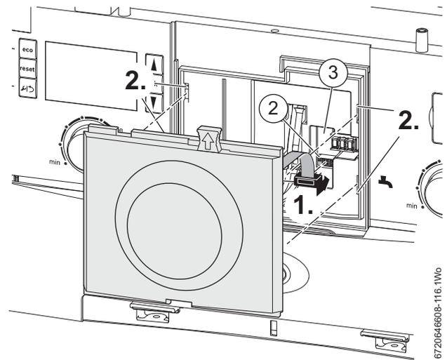
Fig. 50 Connecting the Programmer/Timer
