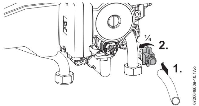
Fig. 84 Draining the boiler
