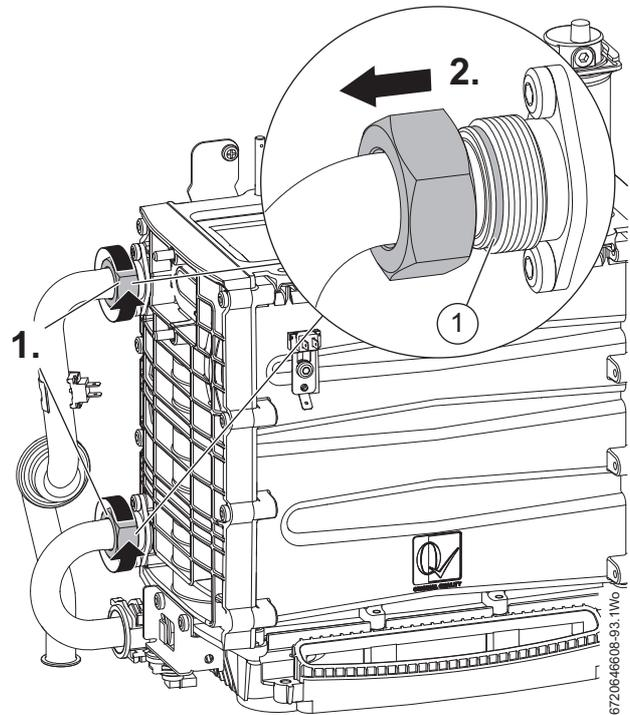
Fig. 104 Heat exchanger disconnection
