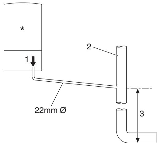
Fig. 4 Disposal to soil vent stack
