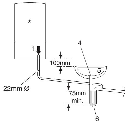
Fig. 5 Disposal to a waste pipe
