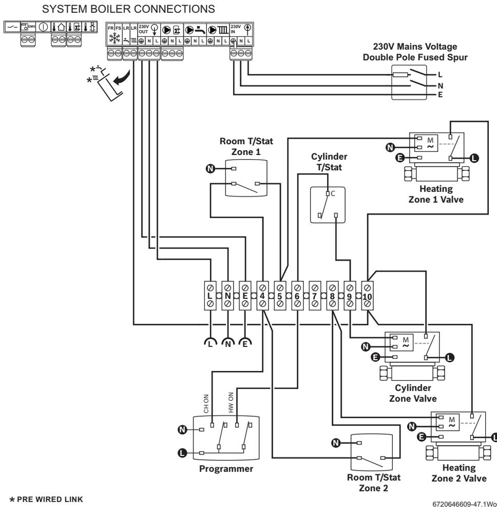
Fig. 52 External controls with vented cylinder
