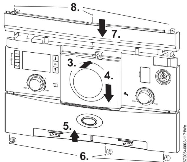
Fig. 51 Fitting the Programmer/Timer
