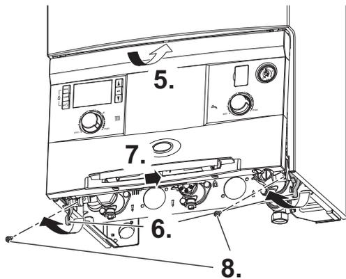
Fig. 65 Fitting case
