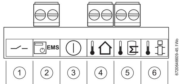
Fig. 47 Low voltage connectors
