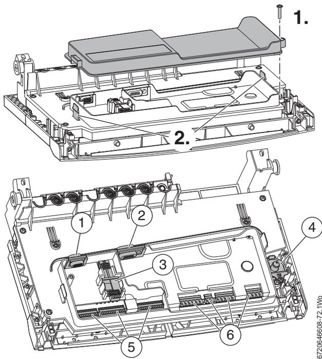
Fig. 117 Access to the cables
