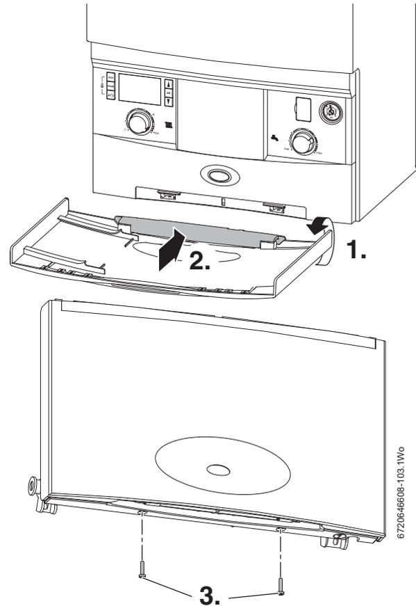
Fig. 66 Installing the fascia flap
