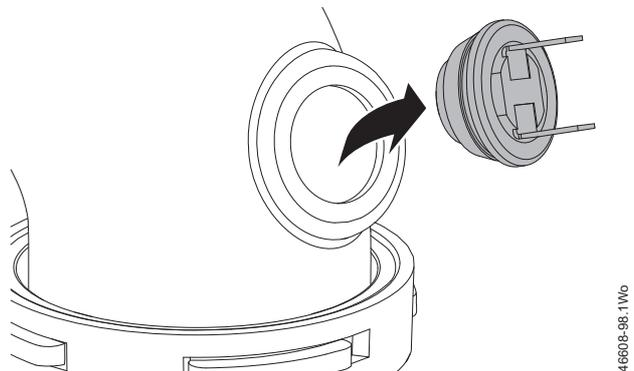
Fig. 88 Flue overheat thermostat
