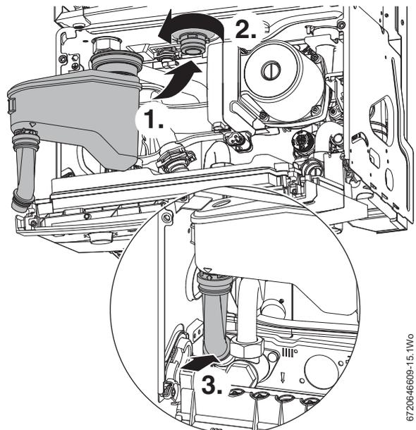
Fig. 78 Fitting siphon
