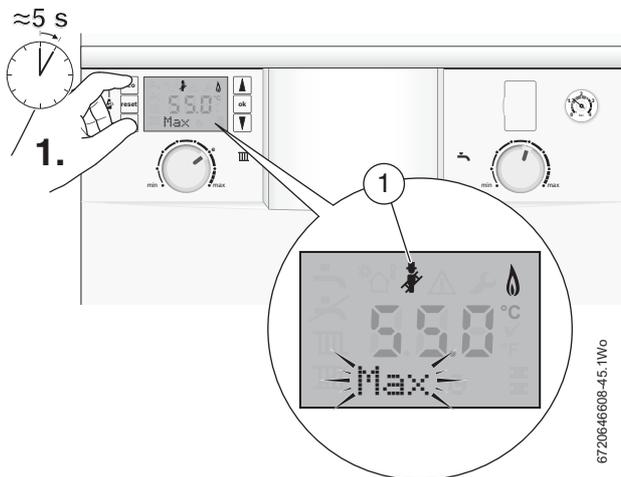
Fig. 63 Setting boiler to maximum
