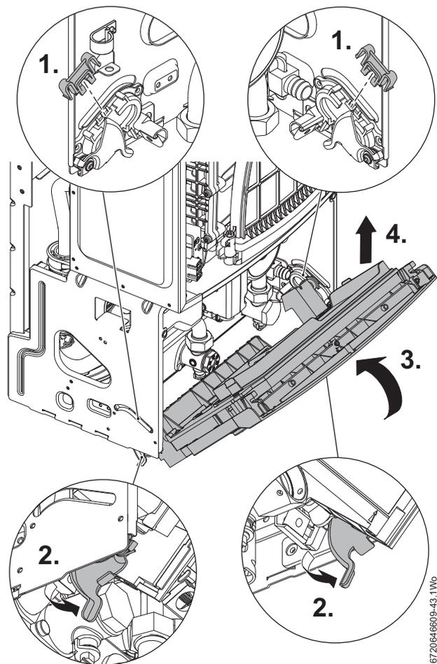
Fig. 118 Removing the controller
