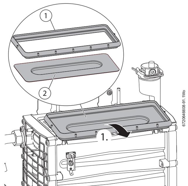
Fig. 102 Burner and gasket
