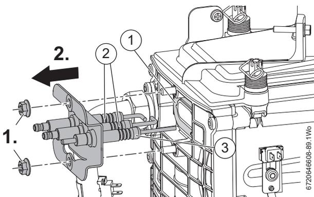
Fig. 100 Electrode assembly
