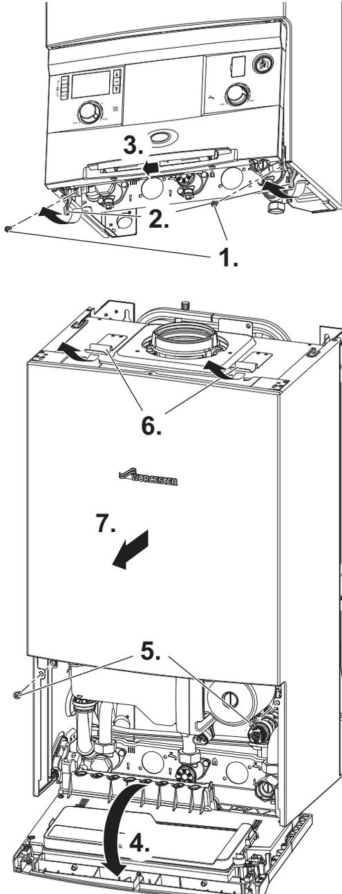
Fig. 83 Removing outer case
