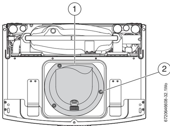
Fig. 41 Aligning the turret
