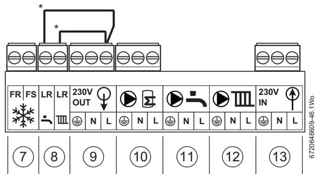
Fig. 48 Mains voltage connectors
