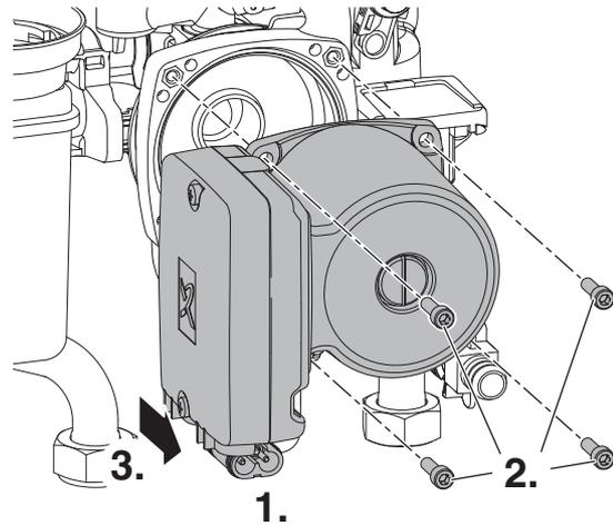
Fig. 107 Pump head removal
