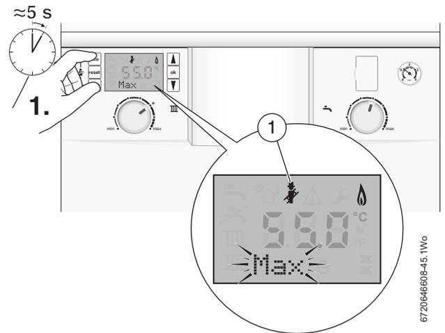
Fig. 60 Setting boiler to maximum
