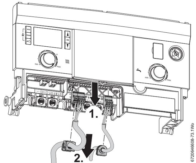
Fig. 116 Disconnect external connections
