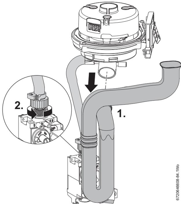
Fig. 95 Combustion air inlet pipe removal
