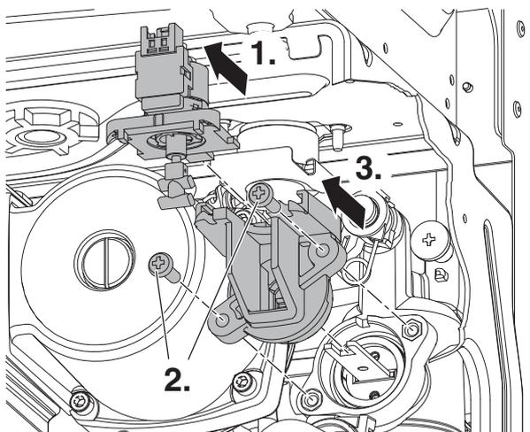
Fig. 106 Diverter valve
