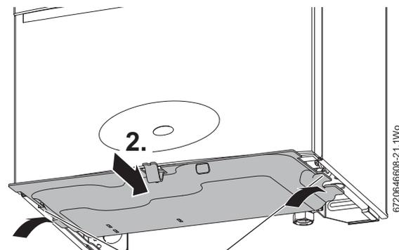
Fig. 67 Bottom panel installation
