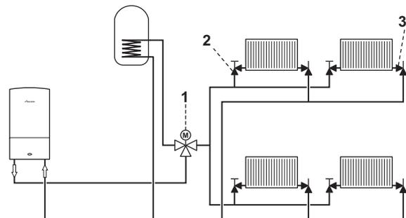
**SYSTEM LAYOUT WITH OPTIONAL INTERNAL DIVERTER VALVE (NOT SUPPLIED WITH BOILER)**
