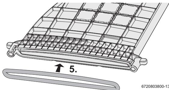
Fig. 94 Tubular style sump seal
