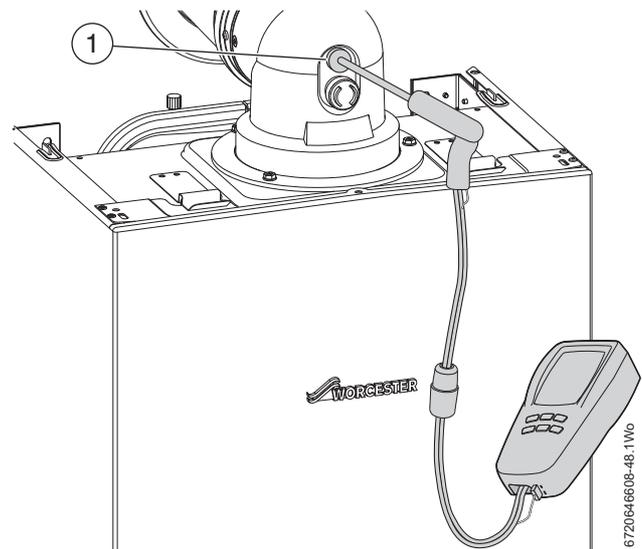
Fig. 71 Flue integrity test
