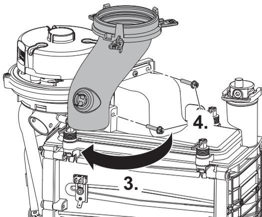
Fig. 96 Fan removal 1
