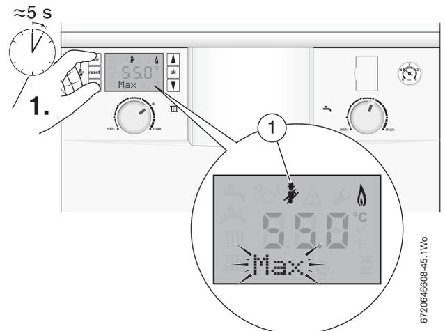
Fig. 73 Set boiler to maximum
