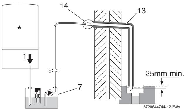
Fig. 9 Condensate pump to external disposal
