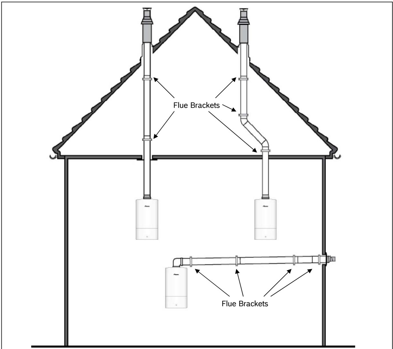
Fig. 1: example of flue supports
