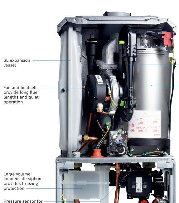
Venturi design provides high, 1:10 modulation range
