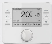
HPC 410 control unit (integrated in the tower and indoor unit)
