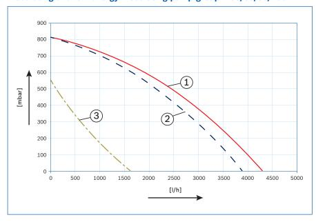
Residual head downstream of the pump group – with and without a non-return valve
