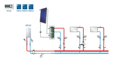
Single GB162 installed with a low loss header.
