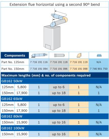
**Note:** The short 0.5m flue extension may be used as an alternative to the standard extension.
