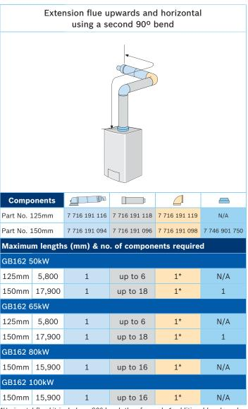
\*Horizontal flue kit includes a 90° bend, therefore only 1 additional bend needs to be ordered.
