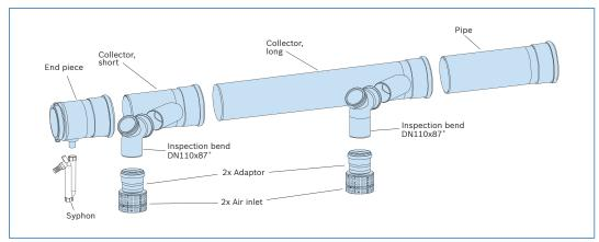
This example shows a typical Worcester flue header kit for a 2 boiler in-line cascade system.
