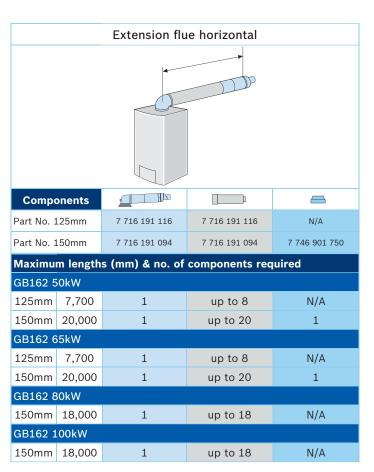
**Note:** The maximum flue length must be reduced by the following amounts for each bend used.
