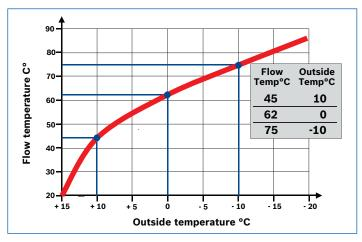
The graph above shows how the heating curve can be modified at any time using the RC35 controller, providing maximum comfort for the user.
