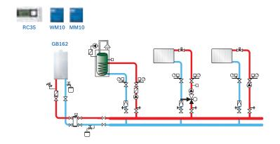
Single GB162 installed with a low loss header. Two heating circuits and DHW are connected to the secondary side of the system. Control is provided completely by RC series equipment.
