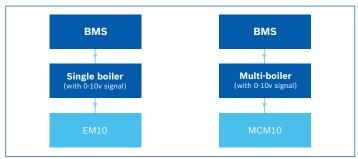
Fig. 1. Compatible BMS controls
