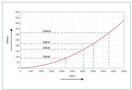
Boiler resistance curveI/h Volume flowmbar Residual head
