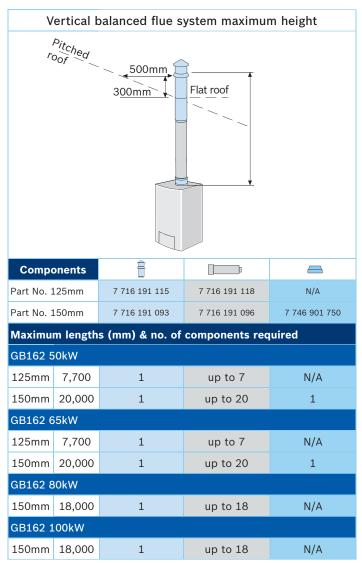
**Note:** The maximum flue length must be reduced by the following amounts for each bend used.
