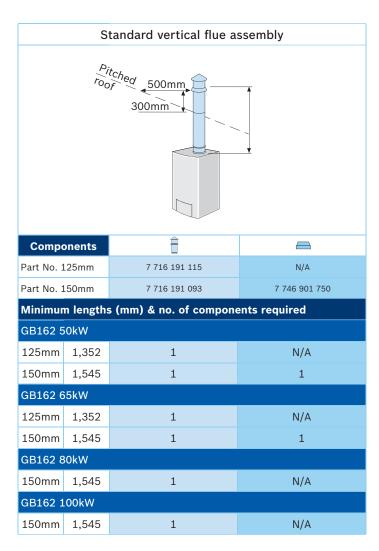
**Note:** The short 0.5m flue extension may be used as an alternative to the standard extension.
