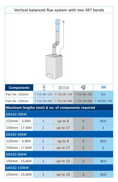
**Note:** The short 0.5m flue extension may be used as an alternative to the standard extension.
