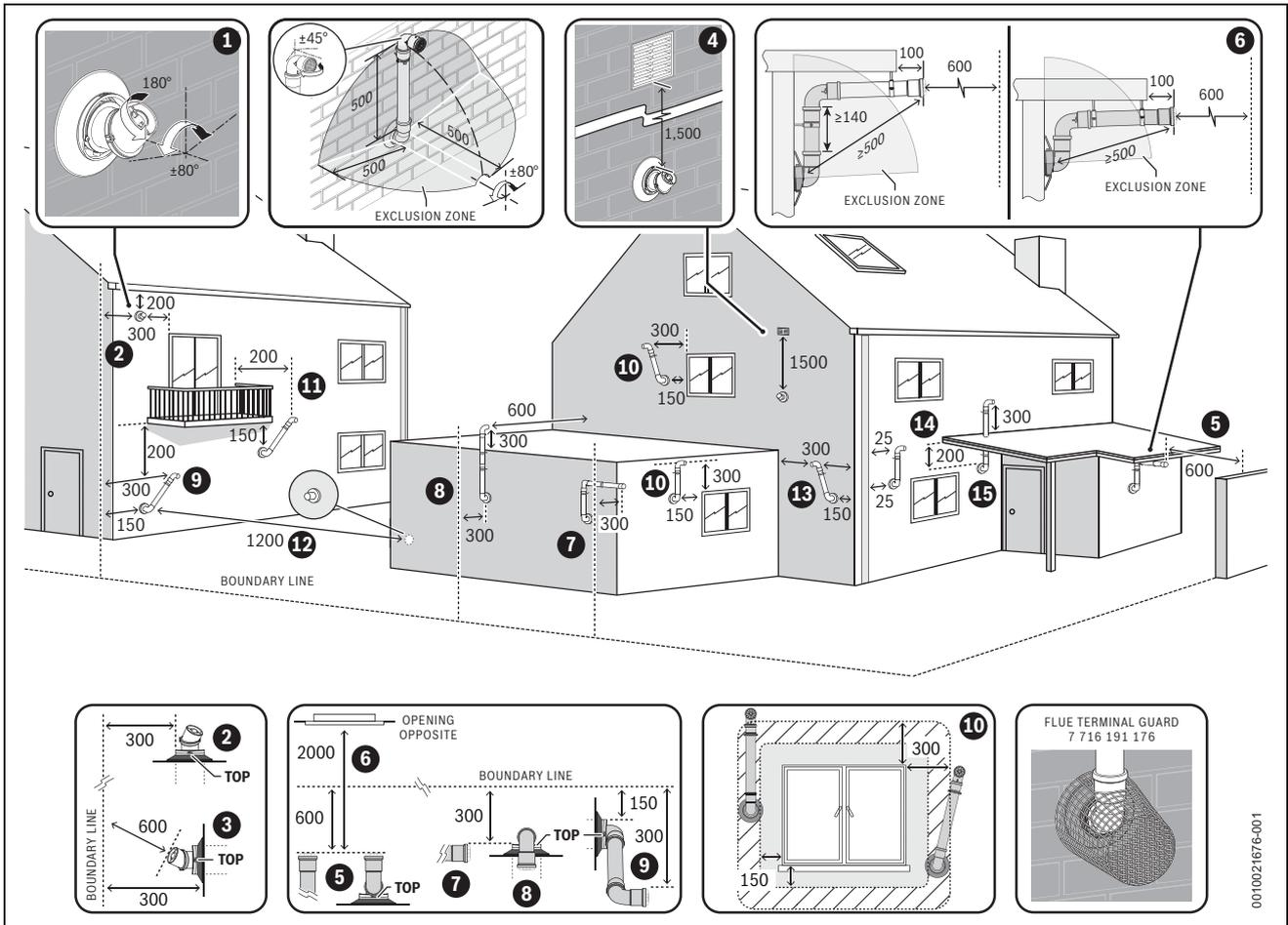
Fig. 32 Plume re-direct and plume management terminal positions
