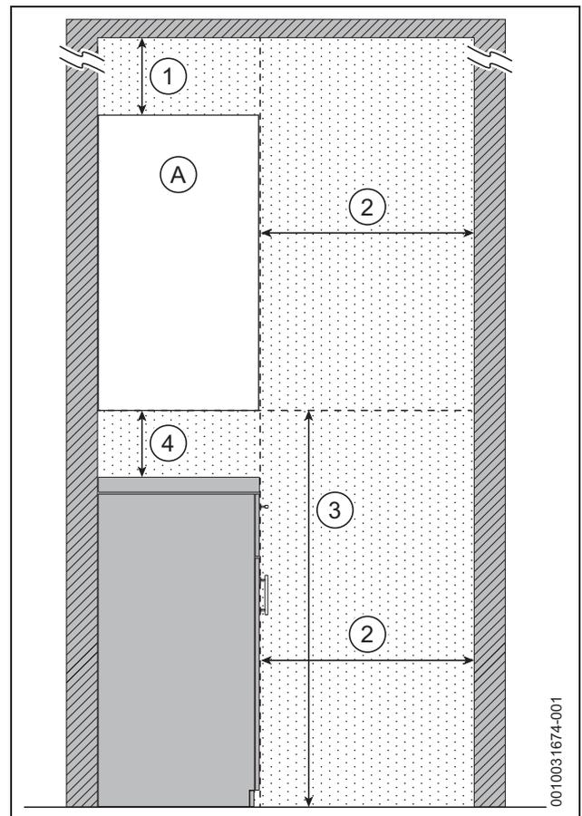
Fig. 13 Reduced front maintenance clearances - Side view
