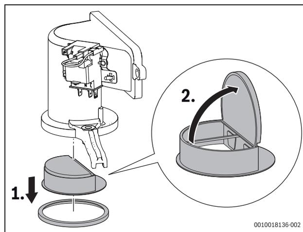
Fig. 86 Non-return valve in the air-gas manifold
