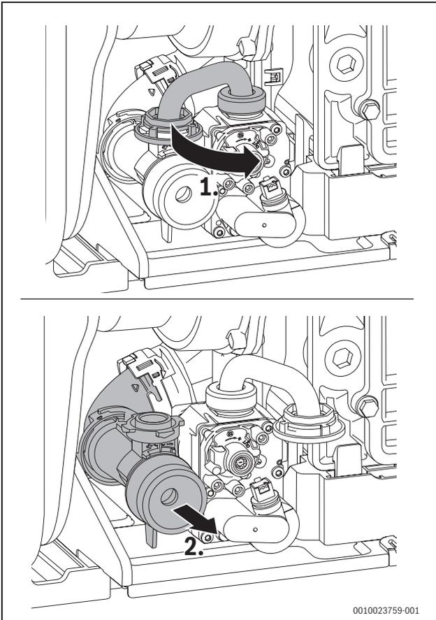
Fig. 87 Venturi removal
