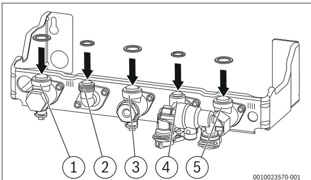
Fig. 47 Fitting the sealing washers
