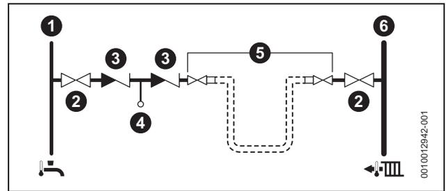
Fig. 8 External filling loop system fill example
