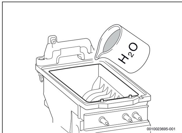
Fig. 92 Pour water into the heat exchanger
