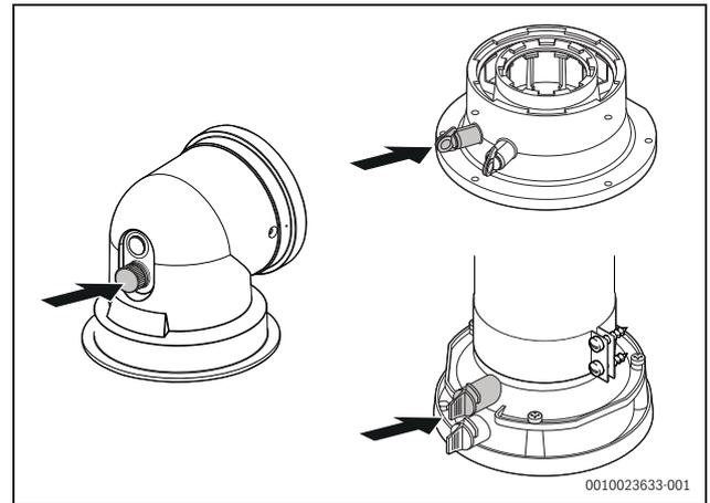
Fig. 103 Flue gas test port
