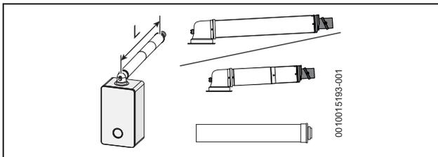
Fig. 19 Horizontal flue option
