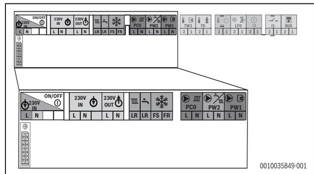
Fig. 60 Power supply (power cables) terminal strip
