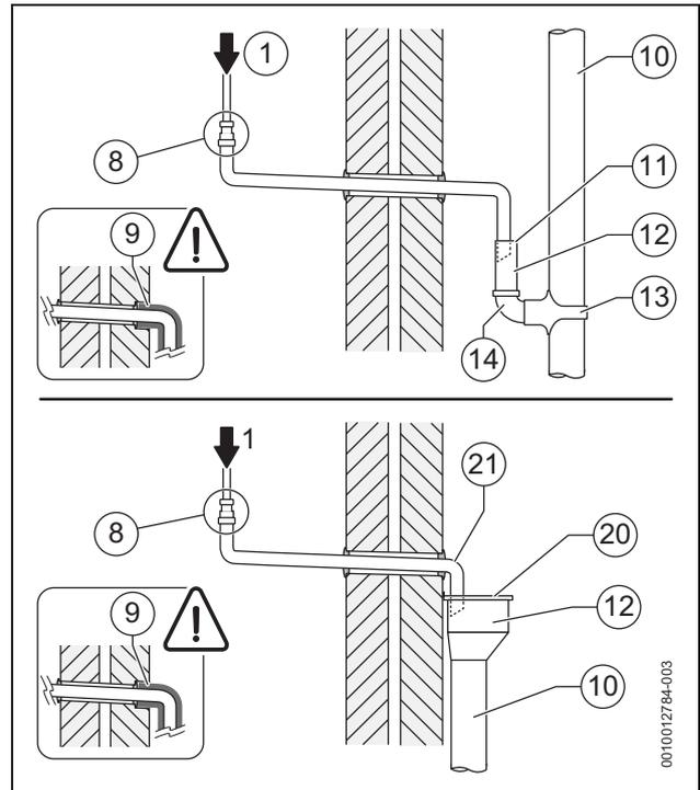
Fig. 37 Disposal into rain water down pipe
