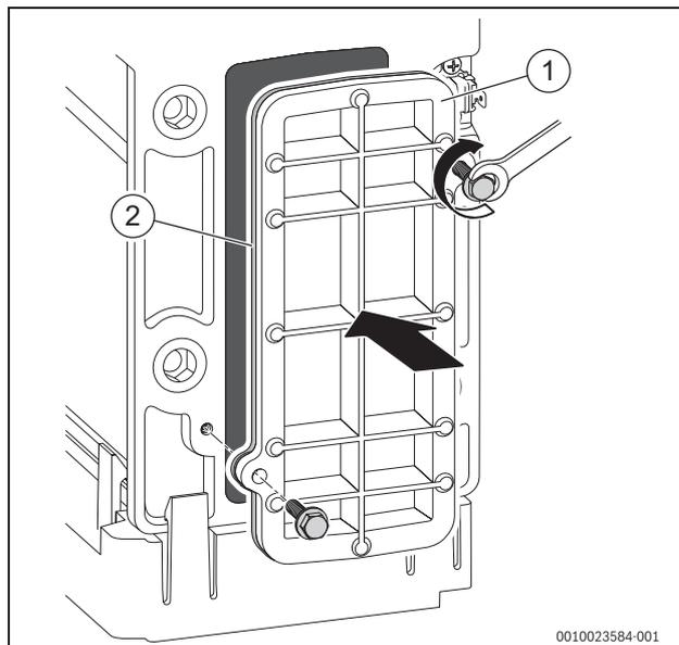
Fig. 94 Re-fitting the access cover
