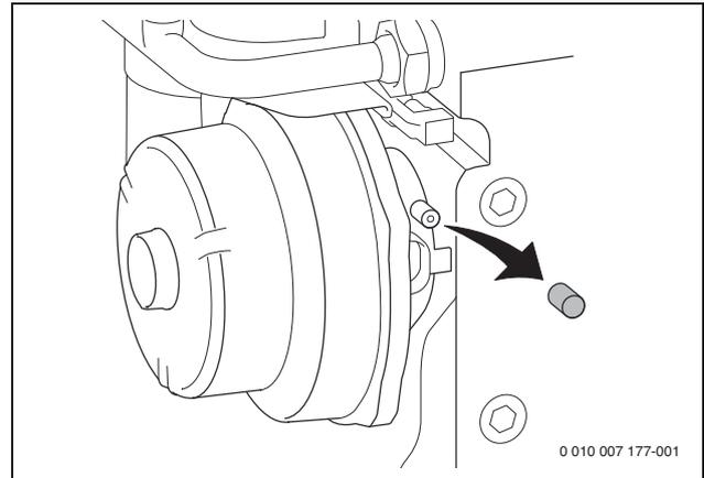
Fig. 81 Test nipple at the mixing device
