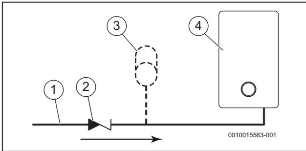
Fig. 9 Mini expansion vessel location
