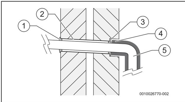
Fig. 36 Additional protection for transition through a wall
