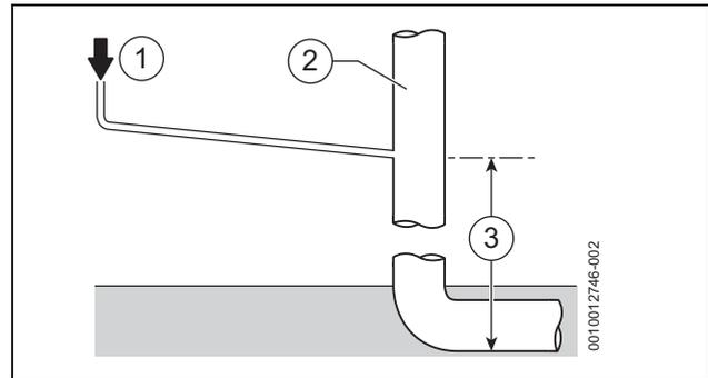
Fig. 33 Disposal to soil vent stack
