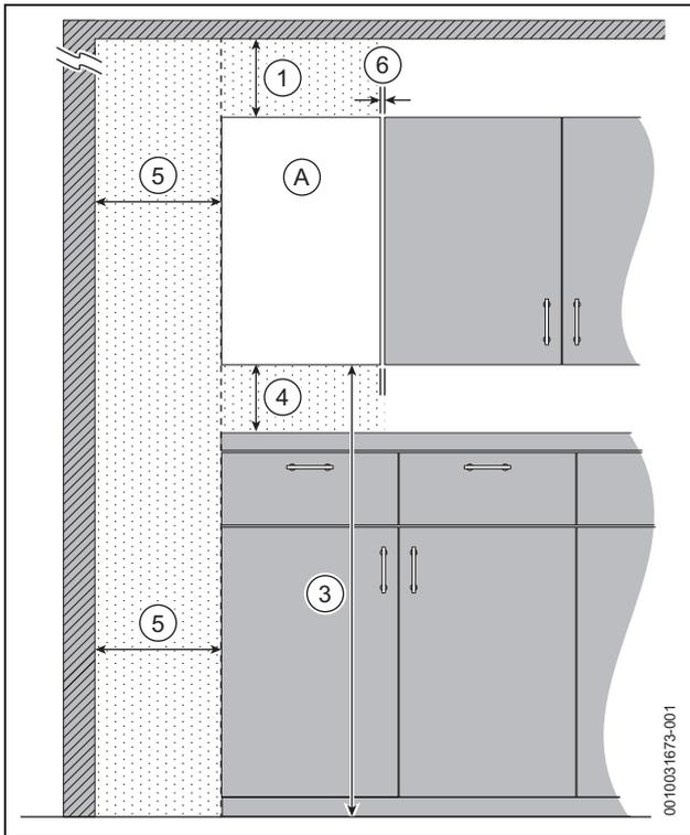
Fig. 14 Reduced front maintenance clearances - Front view
