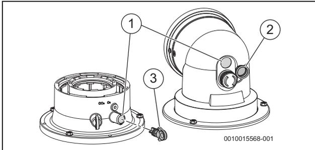
Fig. 76 Flue integrity check test point
