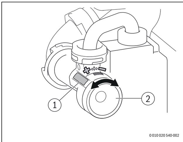
Fig. 102 Setting the adjustable venturi
