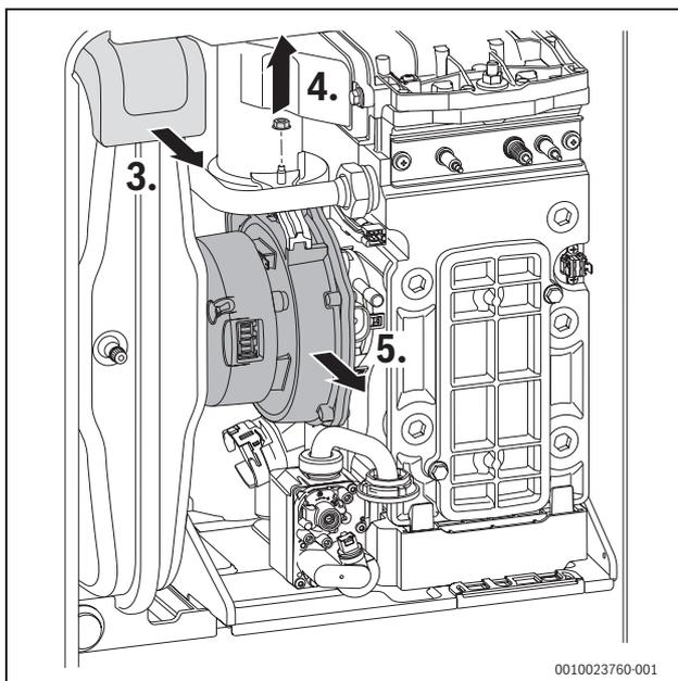
Fig. 88 Fan removal
