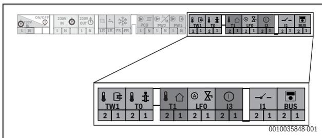
Fig. 61 Low voltage (signal cables) terminal strip
