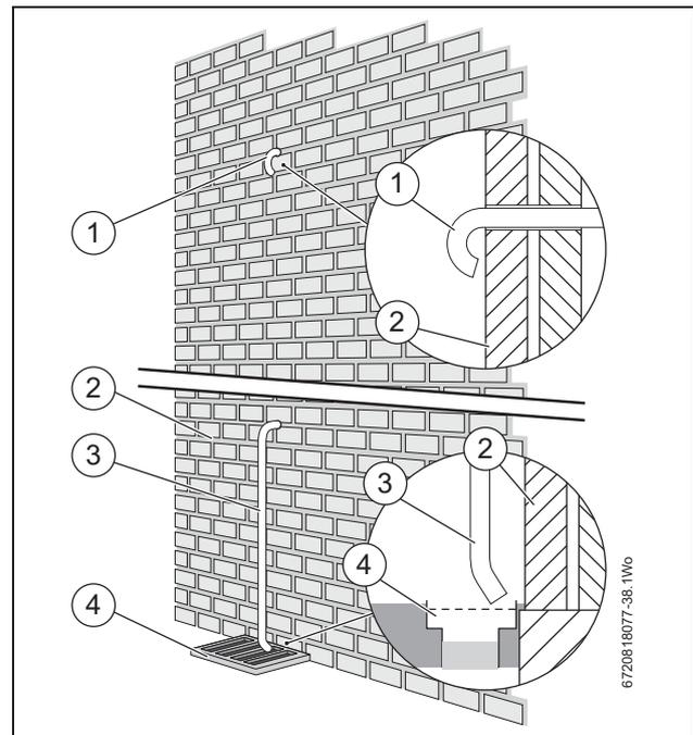
Fig. 41 Pressure relief pipework
