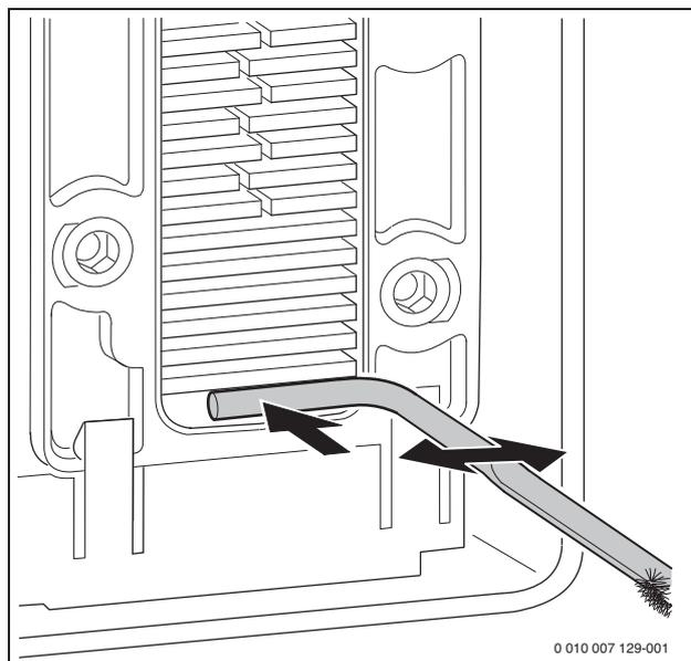
Fig. 93 Cleaning debris
