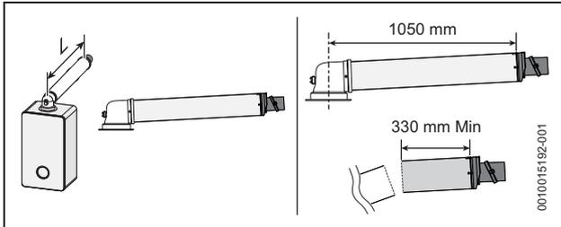
Fig. 18 Horizontal flue option
