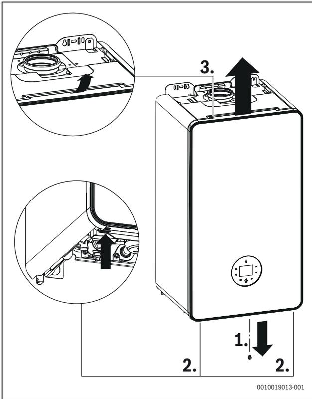
Fig. 80 Removing outer case
