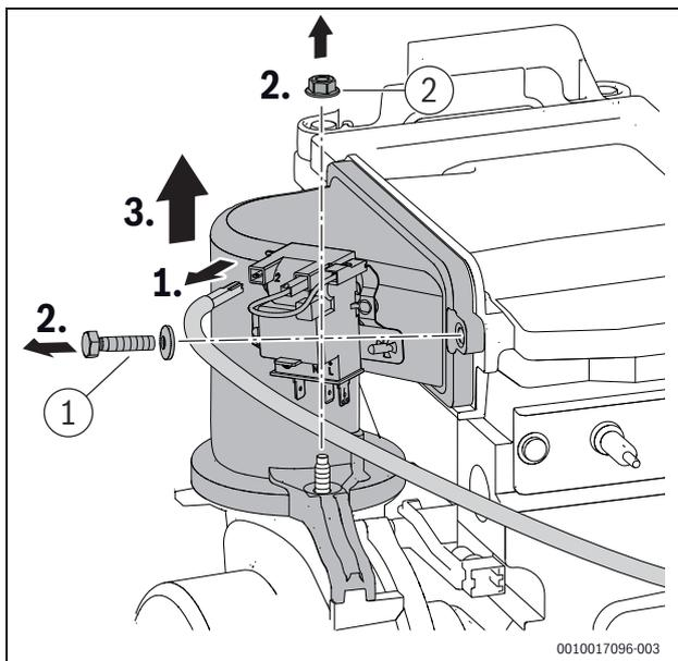
Fig. 85 Removing the air-gas manifold
