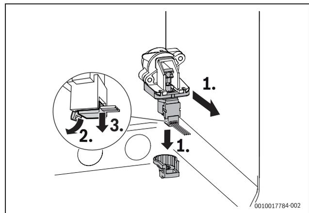
Fig. 113 Removing the motor of the 3-way valve
