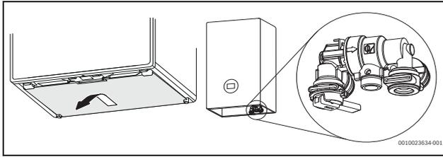
Fig. 67 Enable access to keyless filling link
