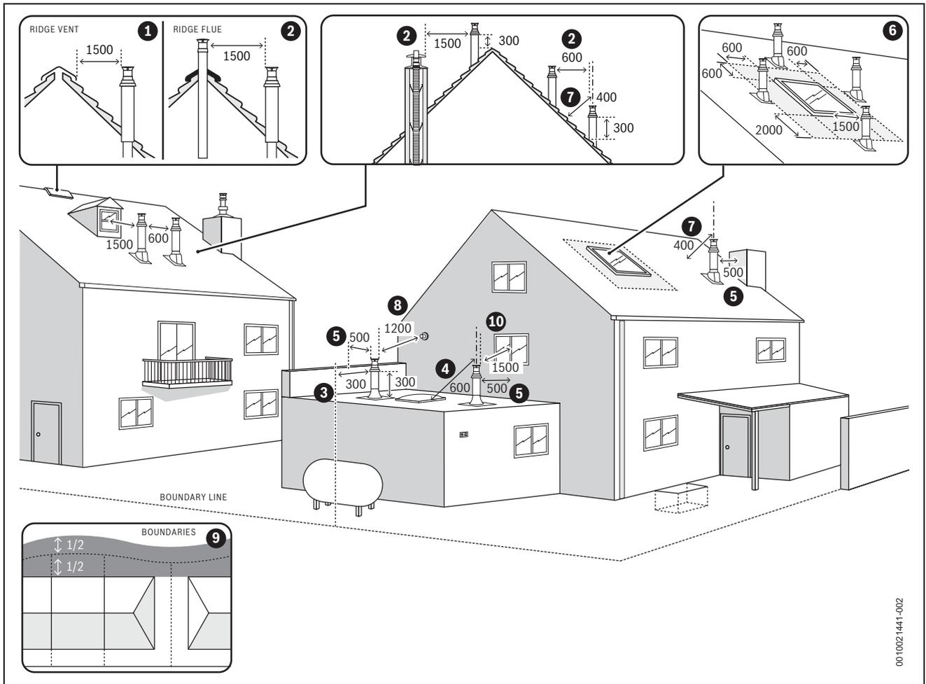
Fig. 30 Vertical flue terminal positions
