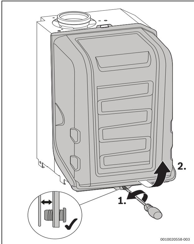
Fig. 101 Removing the combustion cover
