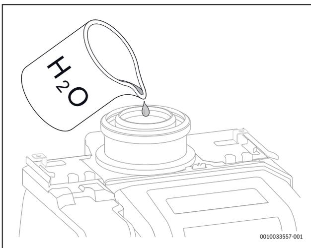
Fig. 54 filling the condensate trap with water
