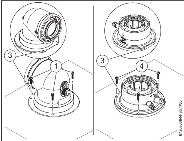
Fig. 57 Flue turret/adaptor connection
