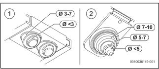
Fig. 53 Adapting the grommets to the cable diameter
