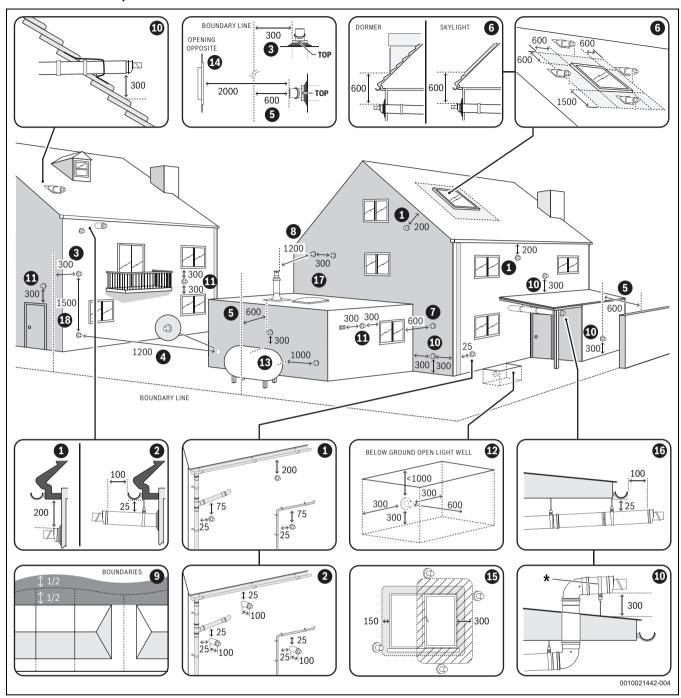
Fig. 38 Horizontal flue terminal positions
