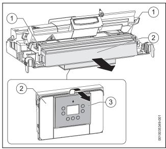
Fig. 98 Control unit removal
