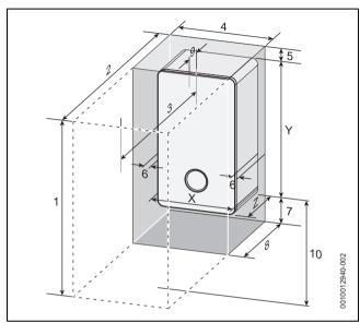
Fig. 17 Appliance minimum clearances
