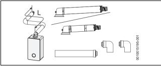
Fig. 26 Horizontal flue option
