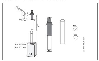
Fig. 33 Vertical flue option
