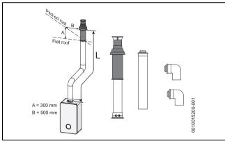
Fig. 32 Vertical flue option
