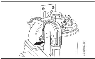
Fig. 70 Test nipple at the mixing device
