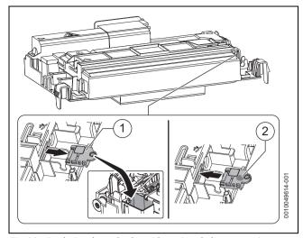
Fig. 62 Replacing the code plug with semi-sealed system variant
