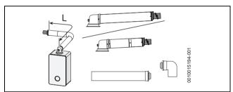
Fig. 25 Horizontal flue option
