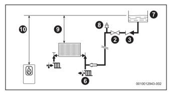
Fig. 16 Semi-sealed system top-up tank fill example
