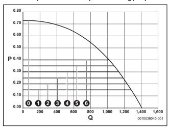
Fig. 99 Pump characteristic maps and pump curves
