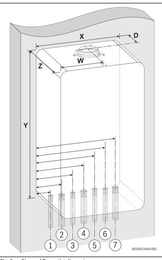
Fig. 2 Pipe and flue outlet dimensions
