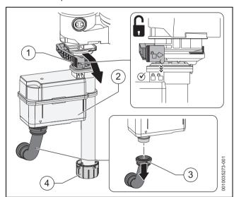
Fig. 79 Removing the siphon
