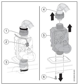
Fig. 89 Removing the gas valve
