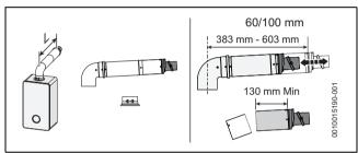
Fig. 21 Horizontal flue option
