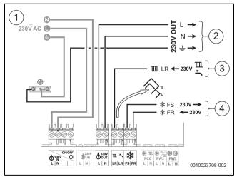
Fig. 59 External controls connections example
