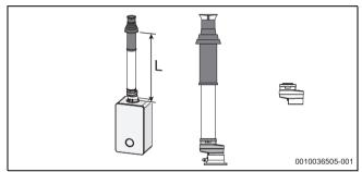
Fig. 34 SimpleSwitch flue adaptor
