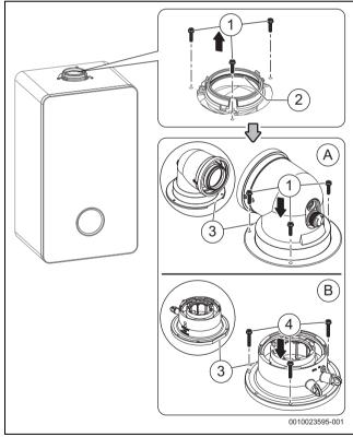
Fig. 51 Flue turret/adaptor connection
