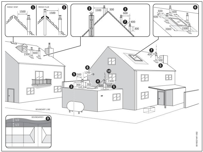
Fig. 37 Vertical flue terminal positions
