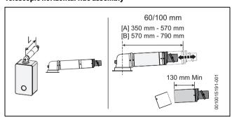
Fig. 22 Horizontal flue option
