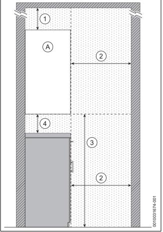
Fig. 18 Reduced front maintenance clearances - Side view
