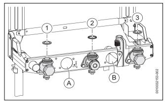
Fig. 46 Fitting the sealing washers
