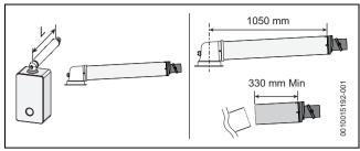
Fig. 23 Horizontal flue option
