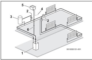
Fig. 12 Cylinder and two heating zones
