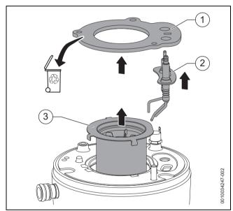
Fig. 74 Removing the burner
