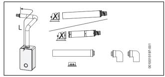
Fig. 28 Horizontal flue option
