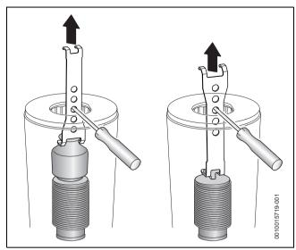
Fig. 75 Remove the top and bottom baffles
