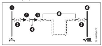
Fig. 15 External filling loop system fill example
