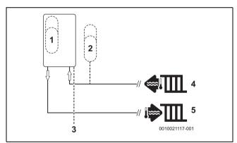
Fig. 4 Additional expansion vessel
