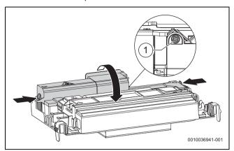
Fig. 60 Opening installer cover
