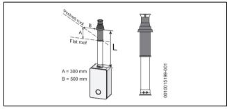
Fig. 31 Vertical flue option
