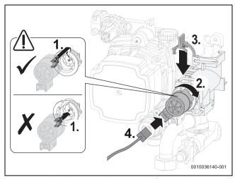
Fig. 88 Installing the motor in the 3-way valve (variant without screws)
