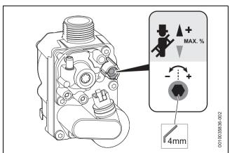
Fig. 83 Setting the CO<sub>2</sub> content
