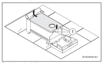
Fig. 41 Removing the front casing
