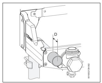
Fig. 44 Condensate drain pipework detail
