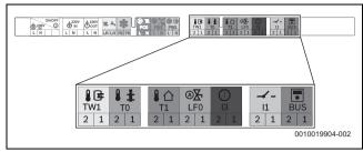
Fig. 58 Low voltage (signal cables) terminal strip
