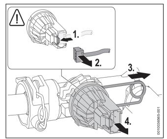
Fig. 93 Pressure sensor removal
