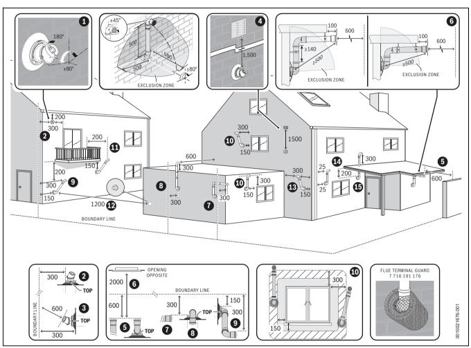
Fig. 39 Plume re-direct and plume management terminal positions
