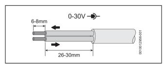
Fig. 55 Low voltage (signal cables) preparation
