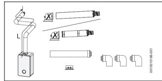
Fig. 29 Horizontal flue option
