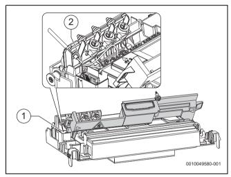
Fig. 61 Semi-sealed system code plug location
