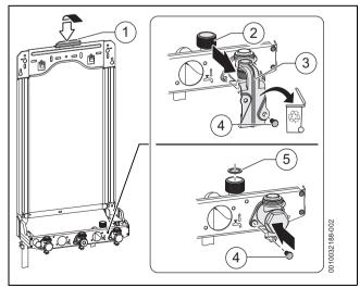
Fig. 47 Wall frame preparation
