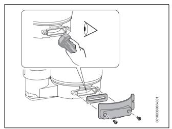
Fig. 78 Checking the heat exchanger for residue
