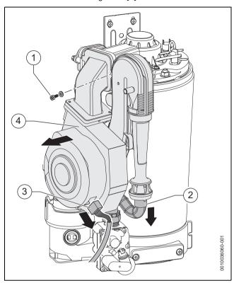
Fig. 71 Removing the fan with mixing unit
