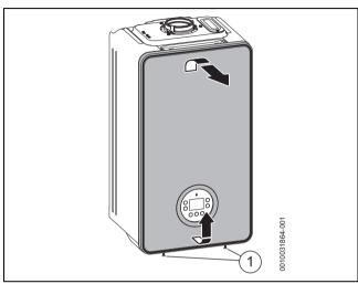
Fig. 69 Removing the front casing
