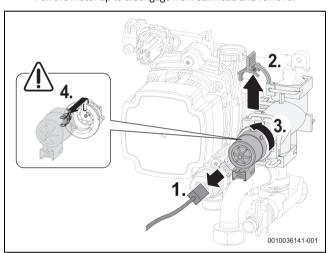
Fig. 87 Detaching the motor from the 3-way valve (variant without screws)
