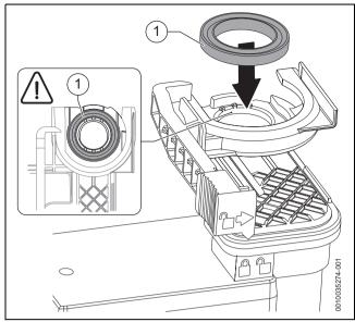
Fig. 80 Replacing the gasket
