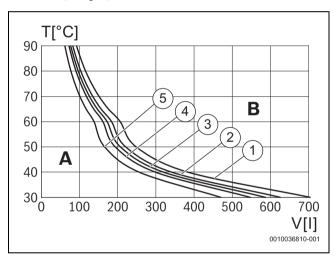
Fig. 5 Curves for the expansion vessel
