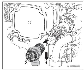
Fig. 92 PRV removal
