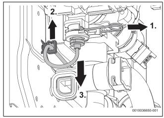
Fig. 95 Rear view of pressure gauge connection
