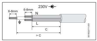
Fig. 54 Power supply (power cables) preparation
