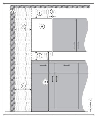
Fig. 19 Reduced front maintenance clearances - Front view
