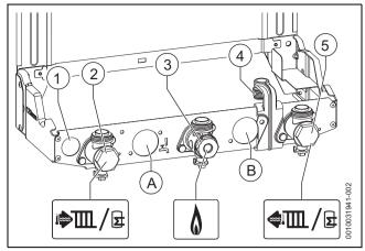
Fig. 43 Connections on the gas and water side
