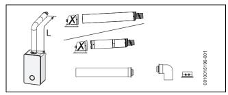
Fig. 27 Horizontal flue option
