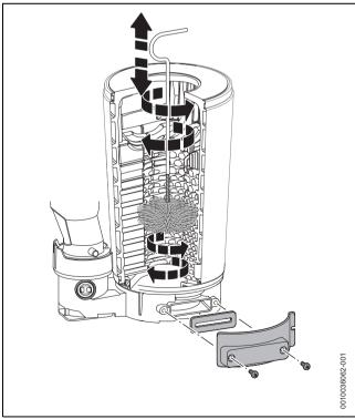
Fig. 76 Cleaning the heat exchanger
