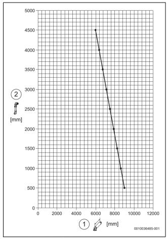
Fig. 35 Plume length to flue length graph
