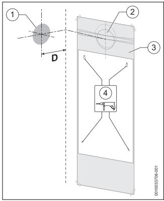
Fig. 42 Wall mounting template
