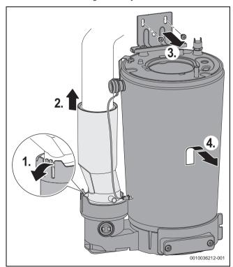
Fig. 86 Removing the heat exchanger assembly
