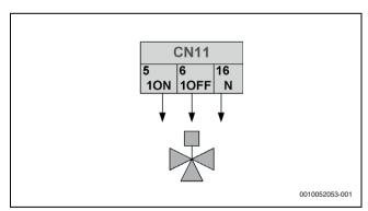
Fig. 77 3-way valve SV1, type 2 control signal
