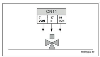
Fig. 85 3-way valve SV3, type 2 control signal
