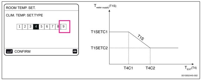
Fig. 149 Customisable curve – outdoor air temperature (T4C1, T4C2) and water supply (T1SETC1, T1SETC2)
