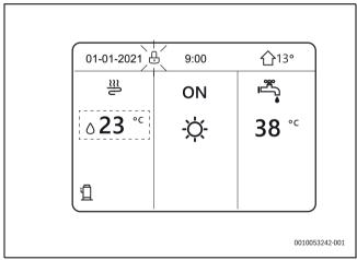
Fig. 159 Locked keypad (flashing)
