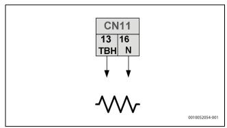
Fig. 78 Booster heater cable HMI configuration, type 2 control signal [TBH] DHW tank booster heater
