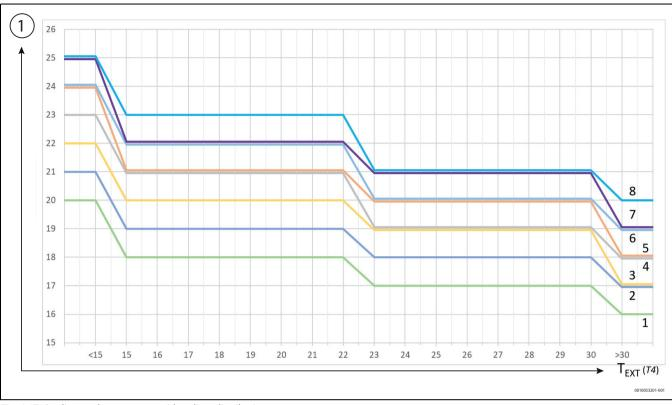
Fig. 147 Cooling mode on systems with radiant distribution
