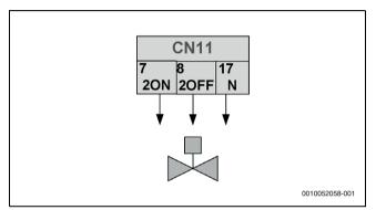
Fig. 82 SV2 2-way valve HMI configuration
