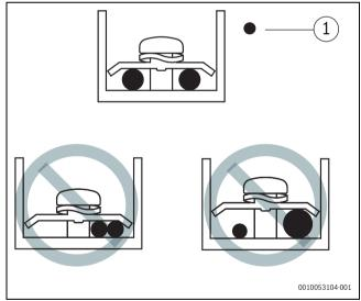
Fig. 69 Danger of overheating due to loose wiring
