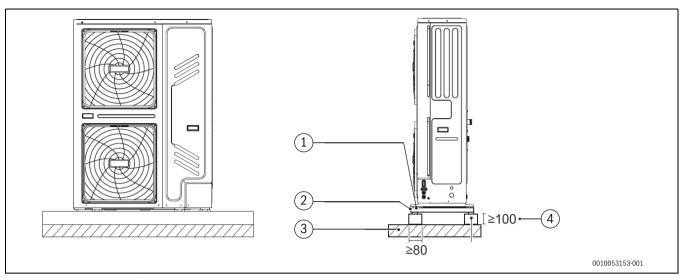
Fig. 42 Secure the unit with foundation bolts
