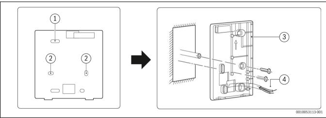
Fig. 97 Installation in electrical box 86
