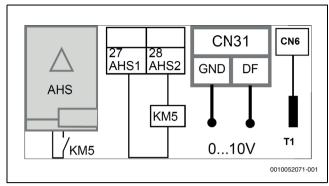
Fig. 91 Additional boiler
