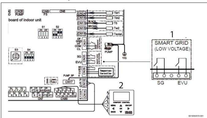
Fig. 92 SMART GRID - Photovoltaic management
