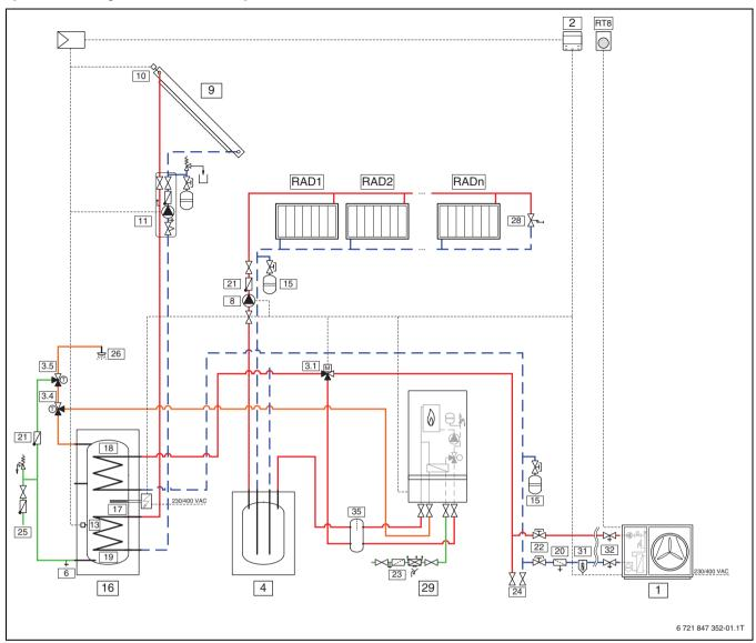
Fig. 21 Outdoor unit with one or many heating circuits, external auxiliary heater, DHW tank and solar (CS2000AWF 4-6 R-S, CS2000AWF 8 -10 R-S, CS2000AWF 12-16 R-S/T)
