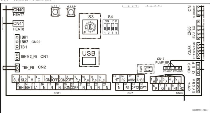
Fig. 72 Connection Terminal Block
