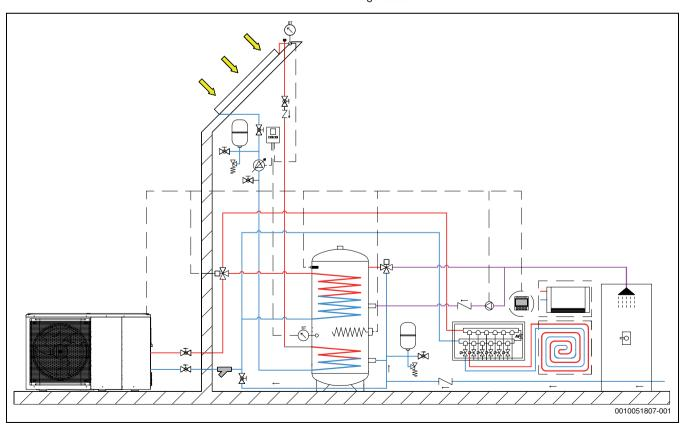
Fig. 51 Water connections
