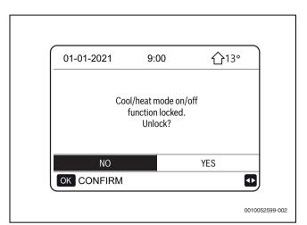
Fig. 219 Unlock COOL/HEAT MODE ON/OFF
