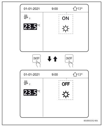
Fig. 167 Radiant panels ON/OFF
