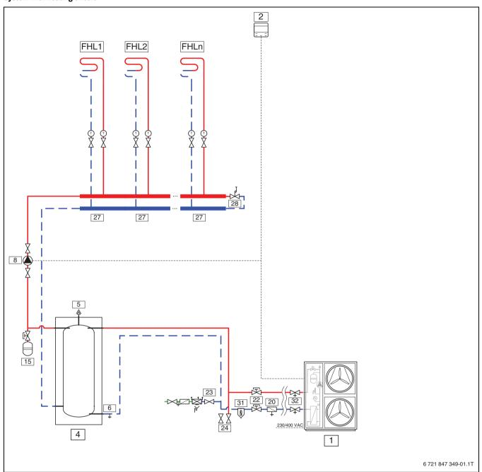
Fig. 18 Outdoor unit with one or many heating circuits (CS2000AWF 18 -30 R-T)
