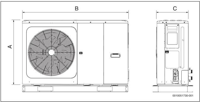
Fig. 32 Sizes CS2000AWF 8 R-S to CS2000AWF 16 R-S/CS2000AWF 16 R-T
