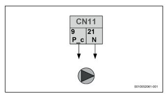
Fig. 84 Zone 2 mixing pump, type 2 control signal
