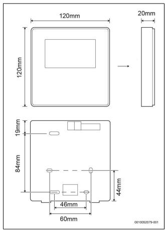
Fig. 94 User interface installation
