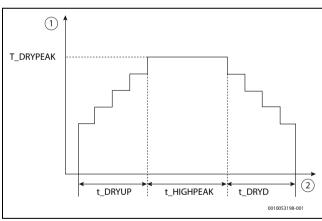
Fig. 142 Drying cycle diagram
