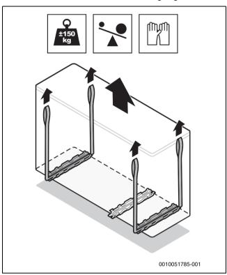
Fig. 44 Placing the unit
