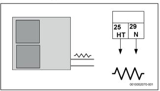
Fig. 90 Antifreeze heater for pipes
