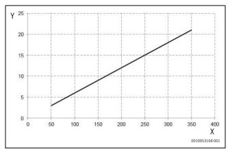
Fig. 55 Total volume for the expansion tank (sizes CS2000AWF 4 R-S to CS2000AWF 16 R-S/CS2000AWF 16 R-T)
