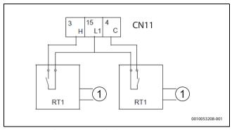
Fig. 102 Zone thermostat - Method C
