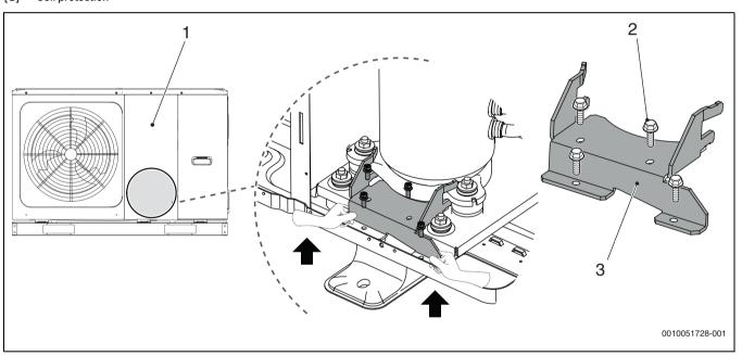
Fig. 30 Removing the transport bracket
