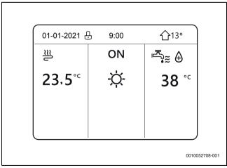
Fig. 187 DISINFECT function is on
