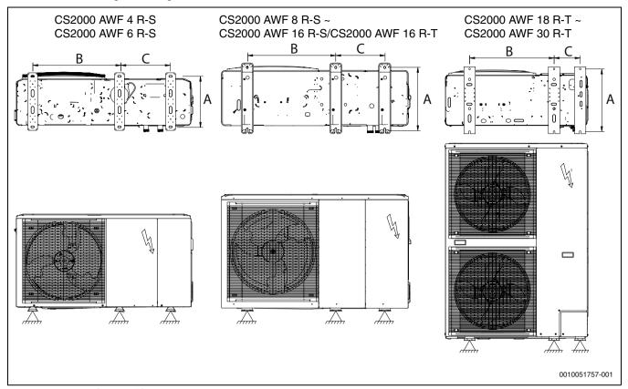
Fig. 41 Dimensions for ground fixing
