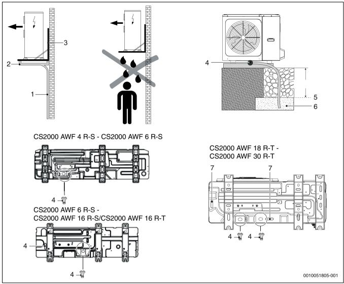
Fig. 48 Condensate drain
