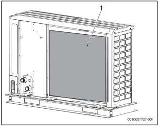
Fig. 29 Removing packaging
