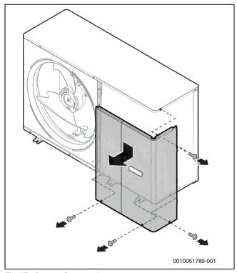
Fig. 47 Remove the protections
