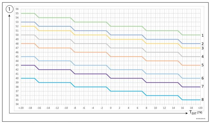
Fig. 145 Heating mode on systems with terminal distribution
