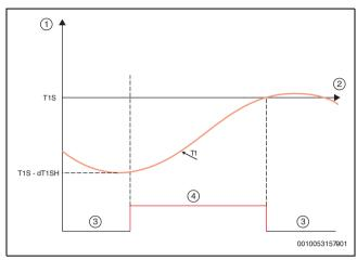
Fig. 124 Heating mode - Water supply temperature (T1)
