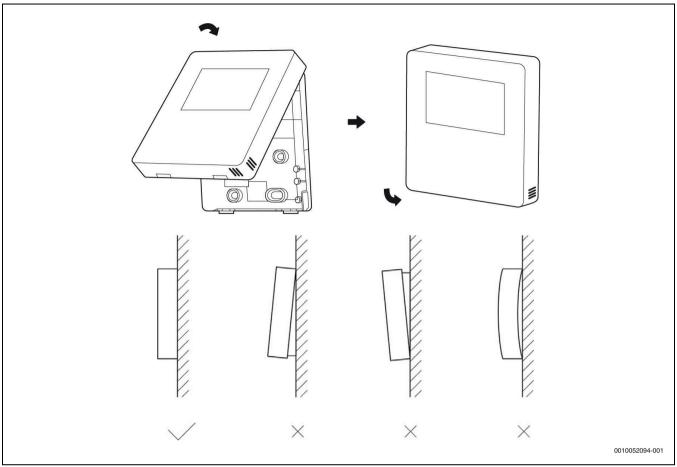
Fig. 99 Installing the front cover
