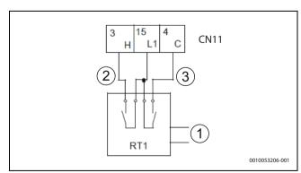
Fig. 100 Zone thermostat - Method A
