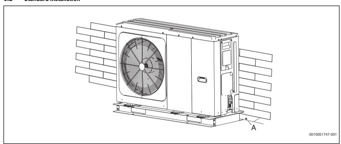
Fig. 34 Standard installation for CS2000AWF 4 R-S ~ CS2000AWF 30 R-T
