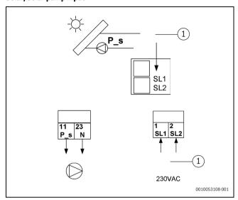
Fig. 75 Solar/Solar pump HMI configuration
