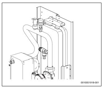
Fig. 59 Filling / topping up with water
