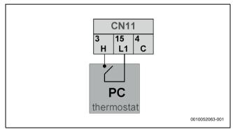
Fig. 86 Room thermostat HMI configuration
