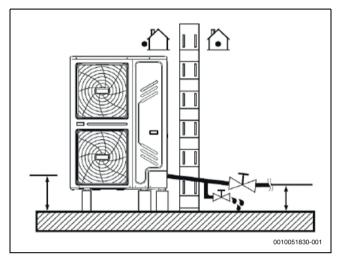
Fig. 53 Water circuit frost protection
