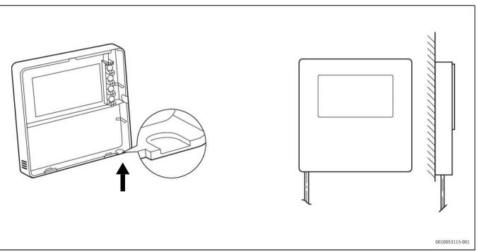
Fig. 95 Positioning of the cable outlet
