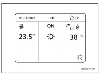
Fig. 190 TANK HEAT function is on
