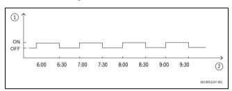
Fig. 193 Pump starting times
