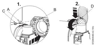
Fig. 53 Refitting the burner
