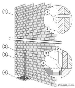
Fig. 20 Pressure relief pipe work
