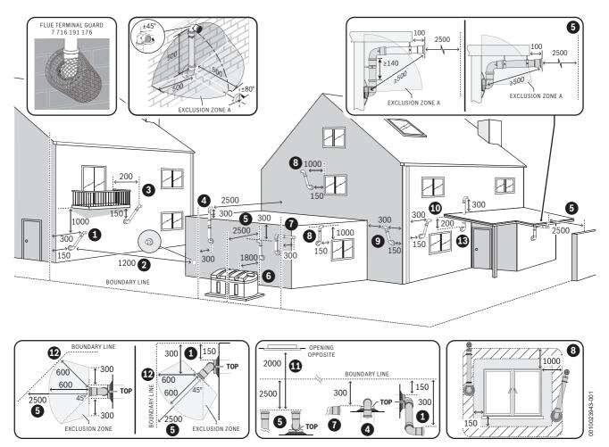
Fig. 28 Plume terminal positions
