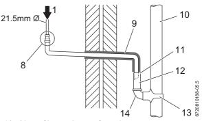
Fig. 16 Disposal into a rainwater down pipe
