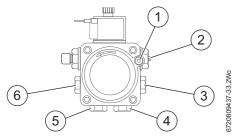
Fig. 64 Oil pump ports/connections
