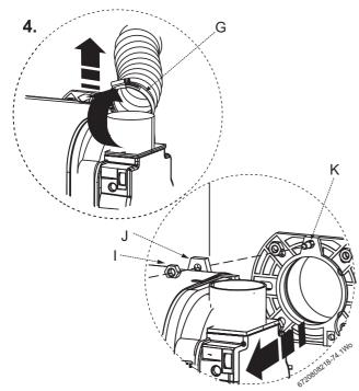
Fig. 78 Burner removal
