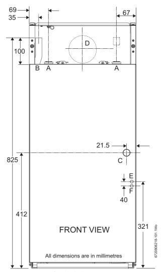
Fig. 31 Front view of Regular boiler pipe connections
