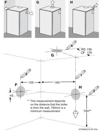
Fig. 35 Flue opening
