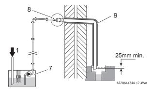
Fig. 18 Condensate pump to external disposal
