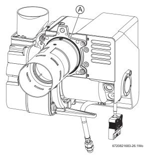
Fig. 52 12/18 Burner O-ring seal shown
