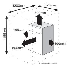
Fig. 21 Installation clearances
