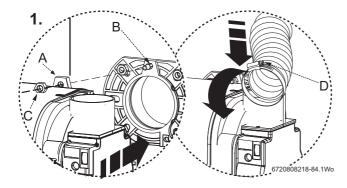
Fig. 89 Refitting the burner
