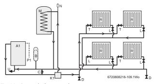
Fig. 11 System boiler system layout
