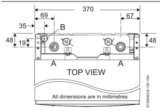
Fig. 30 Top view of Regular boiler pipe connections
