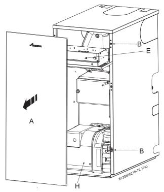
Fig. 75 Access to internal components
