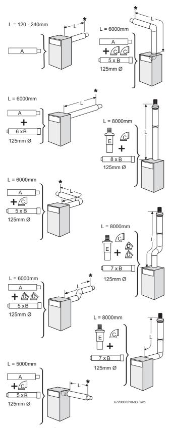
Fig. 27 Room sealed flue options
