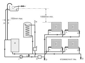
Fig. 9 Regular boiler, open vent layout
