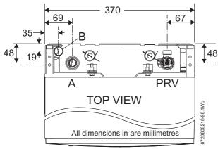
Fig. 32 Top view of System boiler pipe connections
