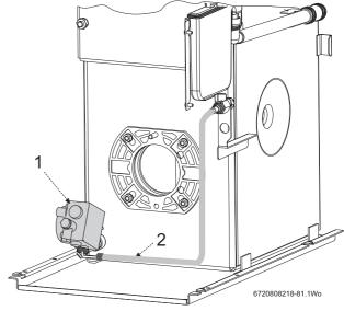
Fig. 90 Oil pump and hose detail
