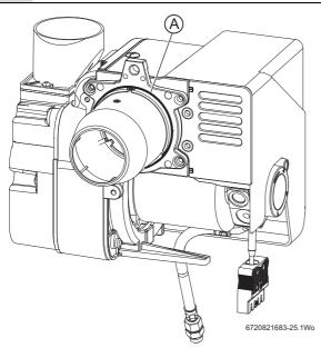
Fig. 88 18/25 and 25/32 Burner O-ring seal shown
