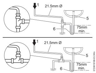
Fig. 14 Disposal to a waste pipe
