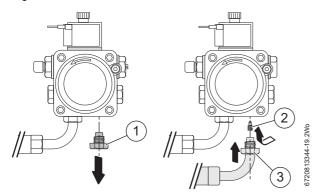
Fig. 51 Converting to double pipe system
