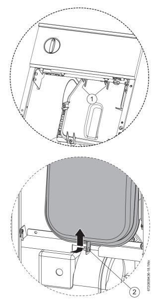
Fig. 73 Expansion vessel location
