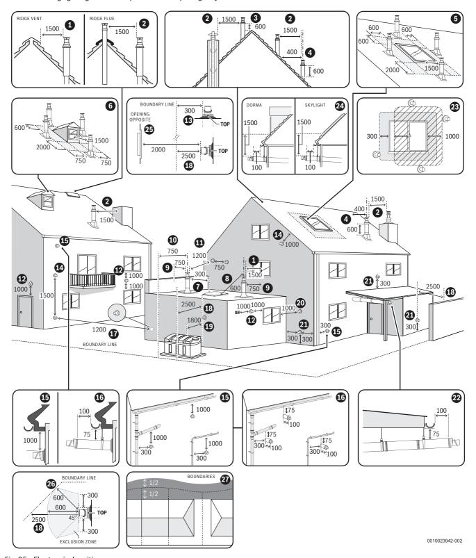
Fig. 25 Flue terminal positions
