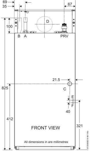
Fig. 33 Front view of System boiler pipe connections
