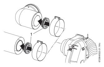
Fig. 40 Flue damper fitting
