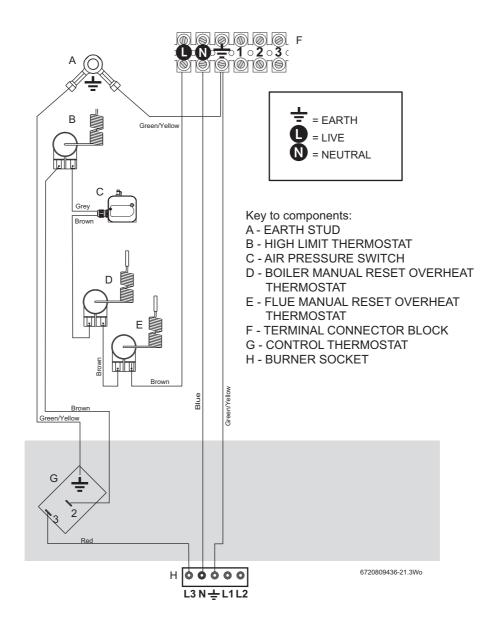
Fig. 56 230V Standard wiring diagram
