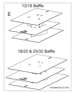
Fig. 43 Baffle arrangement
