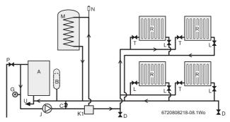
Fig. 10 Regular boiler, system layout
