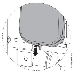
Fig. 76 Expansion vessel removal
