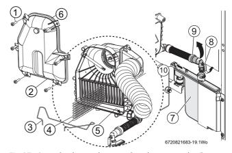
Fig. 87 Secondary heat exchanger and condensate trap detail
