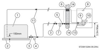
Fig. 6 Double pipe feed
