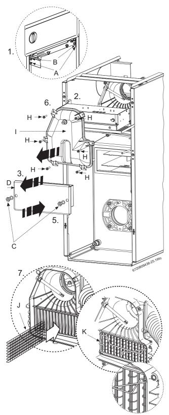
Fig. 42 Combustion chamber
