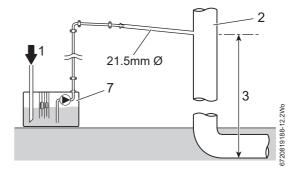
Fig. 15 Condensate pump disposal
