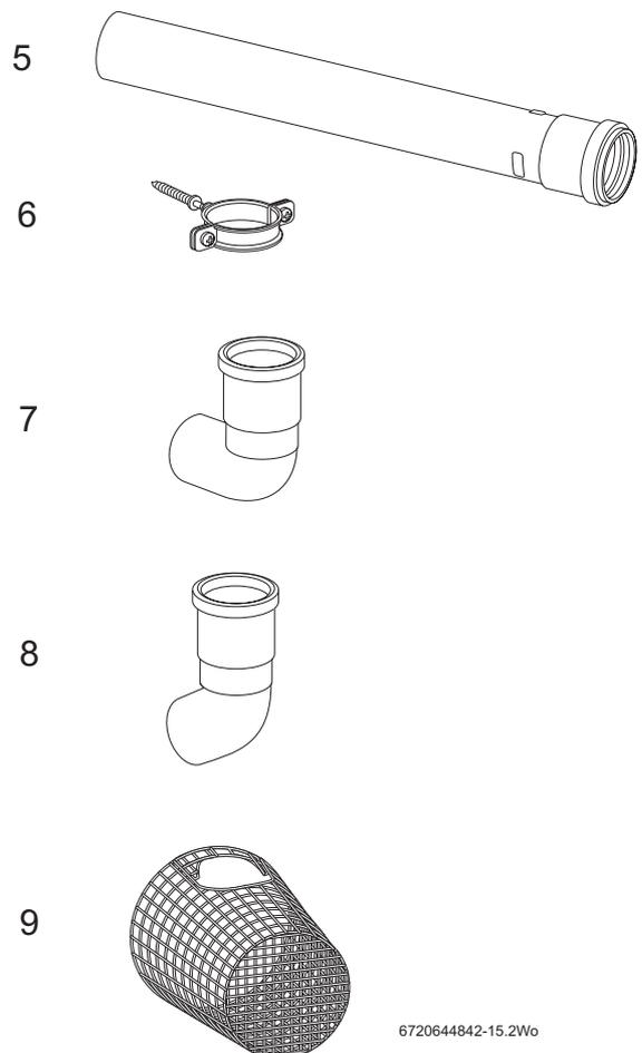
Fig. 29 Plume management extension components
