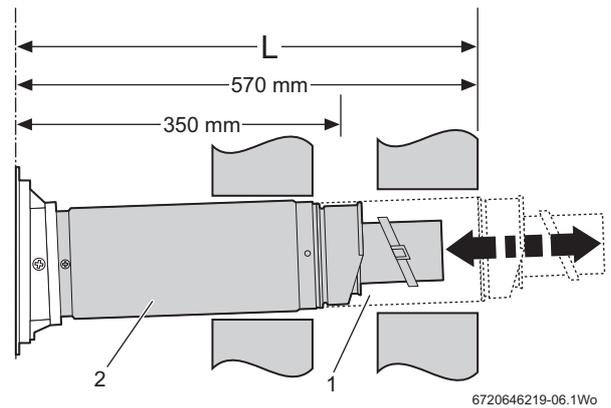
Fig. 7 Standard telescopic flue
