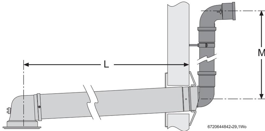
Fig. 35 Effective lengths L and M
