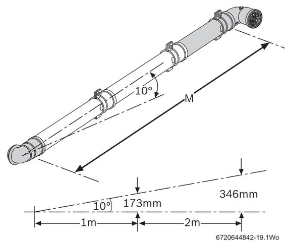
Fig. 34 Plume management with straight extension
