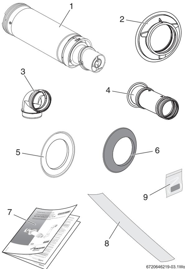
Fig. 1 Telescopic flue components
