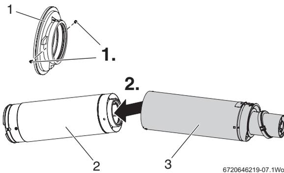
Fig. 8 Reducing the telescopic terminal
