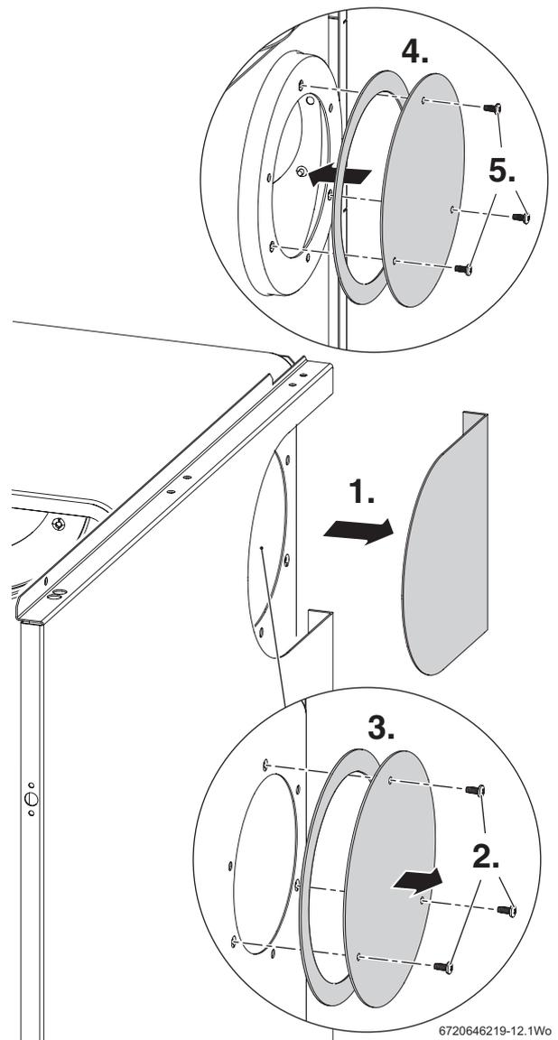
Fig. 14 Converting from rear to side flue outlet
